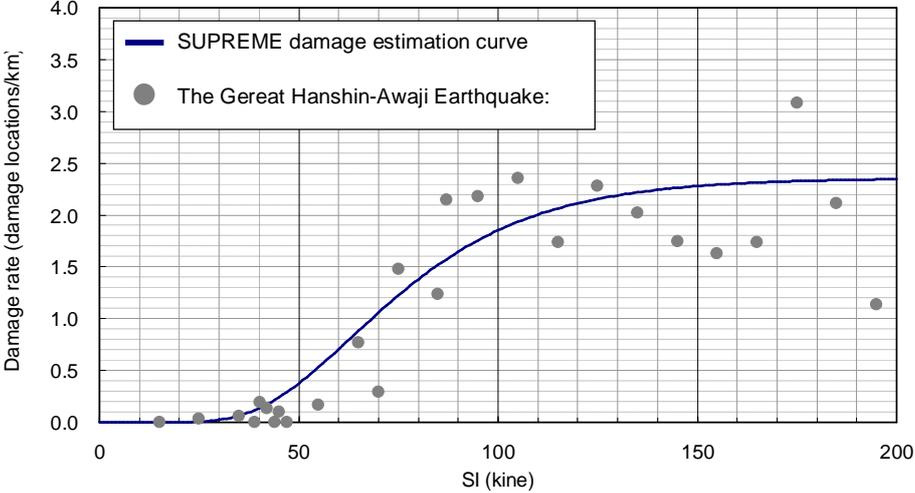
**Figure 2.** Damage Estimation Curve of SUPREME
