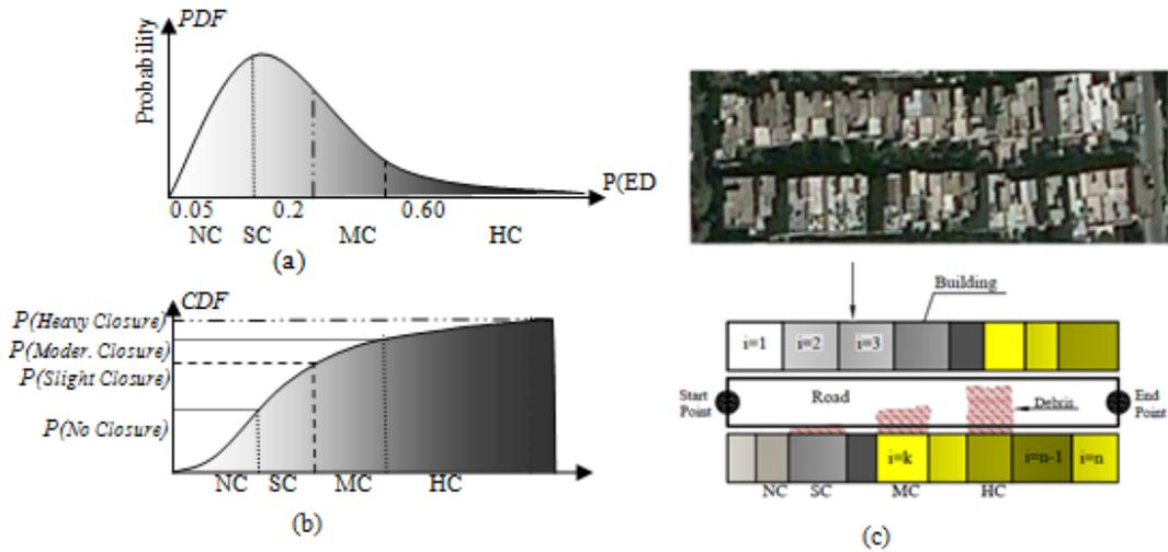
**Figure 4.** Probability distribution of extended debris for each building bordering a road section
