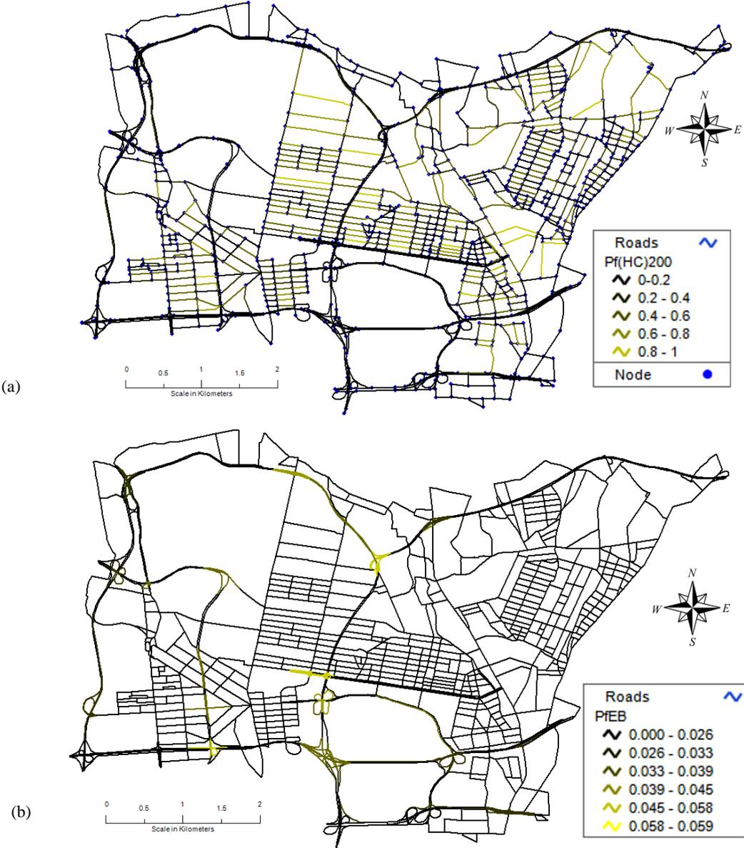
**Figure 6.** Probabilistic map showing the probability of at least one heavy closure (*HC*) on each road segments for event with 200 years return period: a) cumulative effect of both building debris and damaged bridges, b) effect of damaged bridges only
