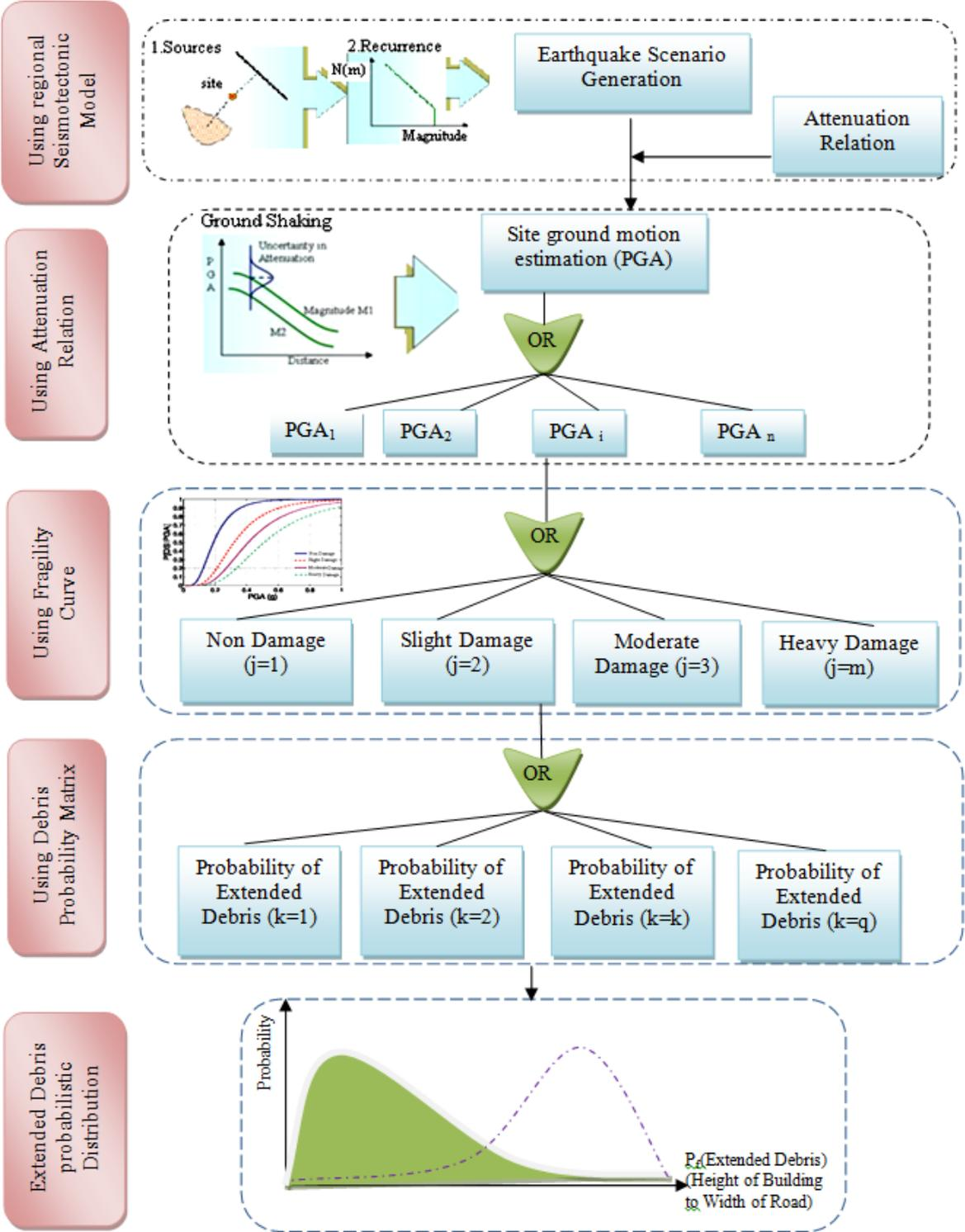
**Figure 3.** Logic tree algorithm to estimate probabilistic distribution of extended debris on urban roads caused by building damage. In this framework an earthquake may results in  $n$  levels of PGA at a site, each resulting in  $m$  stages of structural damages on a building, each damage level resulting in  $q$  stages of road closures.
