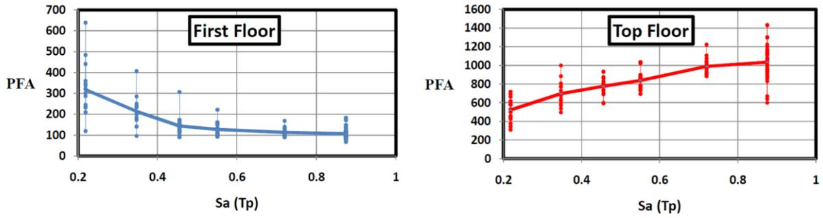
Figure. 4.3: Average  $PFA_e$  for the first and top floors of a 7-story frame subjected to 15 far-field records.
