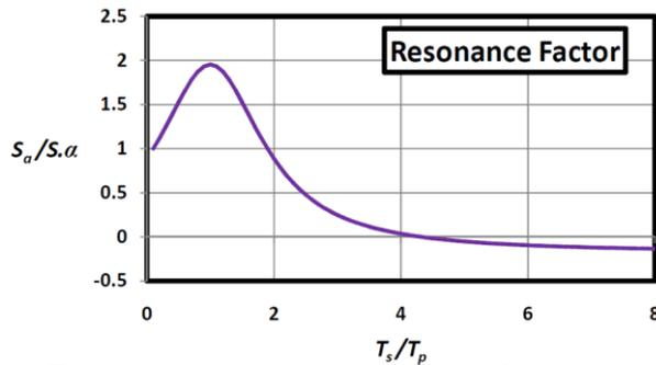
Figure. 7.1: Resonance factor according to Eurocode 8 formulations.
