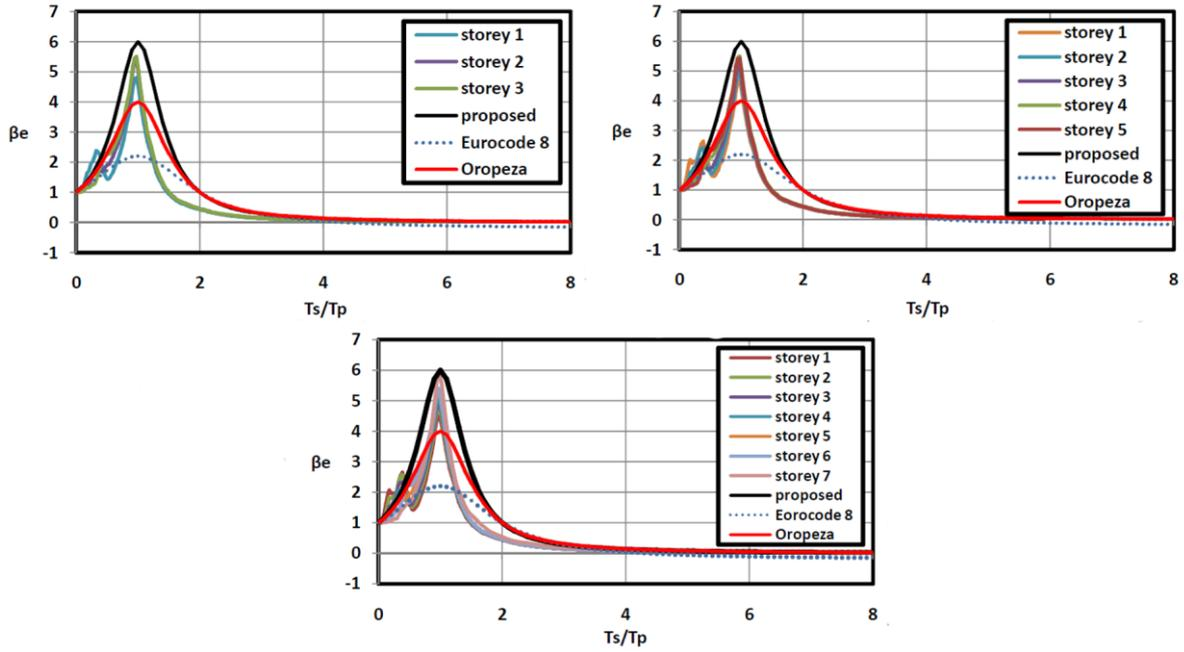
Figure. 7.2: Average  $\beta_e$  for 3, 5, and 7-story frames with the period of 0.67 sec. subjected to 15 records.
