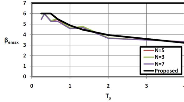
Figure. 7.3: Comparing  $\beta_{emax}$  of 3, 5, and 7-story structures subjected to 15 far-field records.
