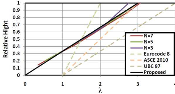
Figure. 6.1: Average amplification factors for 3, 5, 7-story elastic structures with a period of 0.67 second.
