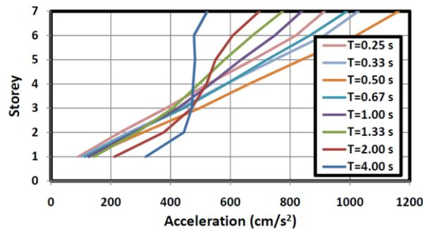
Figure. 4.1: Peak floor acceleration of 7-story elastic frames with eight different periods.
