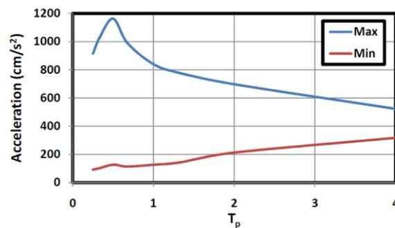
Figure. 4.2: Peak floor acceleration of seven-story elastic frames with different periods.
