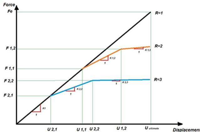
Figure. 3.2: Force-displacement curve for producing a frame with inelastic behaviour.
