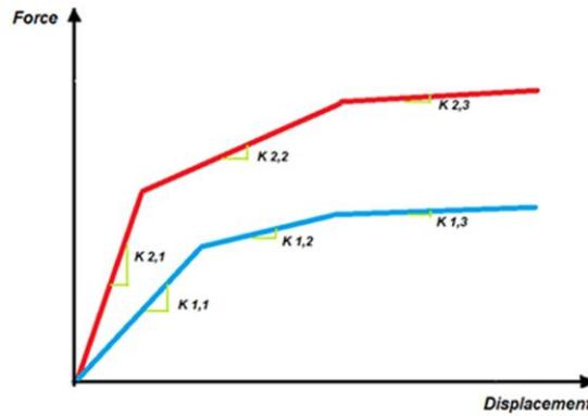
Figure. 3.1: Method of changing period of structure by keeping stiffness ratios constant.
