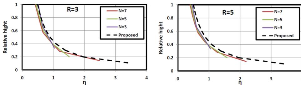
Figure. 8.1: Average parameter  $\eta$  in 3, 5, and 7-story inelastic structures with the period of 0.67 sec. and reduction factors ( $R$ ) of 3 and 5, subjected to 15 far-field records.
