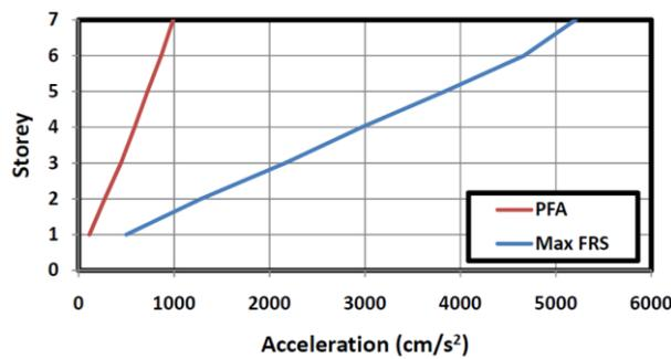
Figure. 5.2:  $PFA_e$  and maximum  $FRS_e$  of a 7-story frame with a period of 0.67 second.
