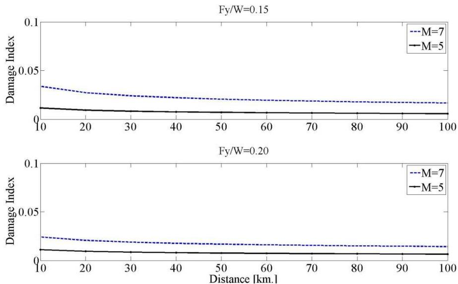
**Figure 4.** Attenuation of the damage spectra with source-to-site distance for structures with ductility=3 and  $T= 1.0$  sec.
