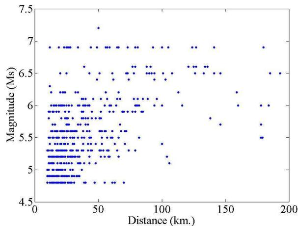
**Figure 1.** Distribution of the magnitude and distance of ground motion records on rock and stiff soil
