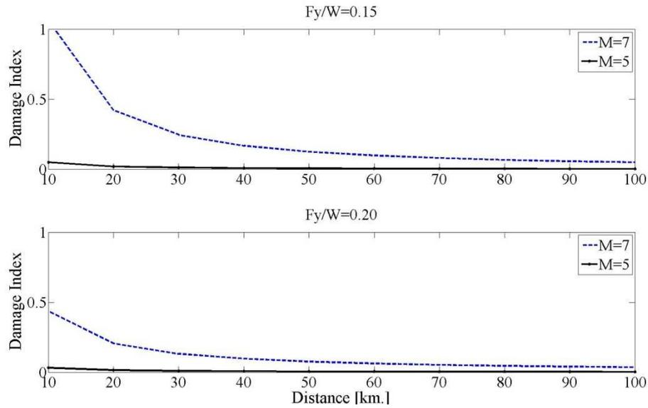
**Figure 3.** Attenuation of the damage spectra with source-to-site distance for structures with ductility=3 and  $T= 0.3$  sec.
