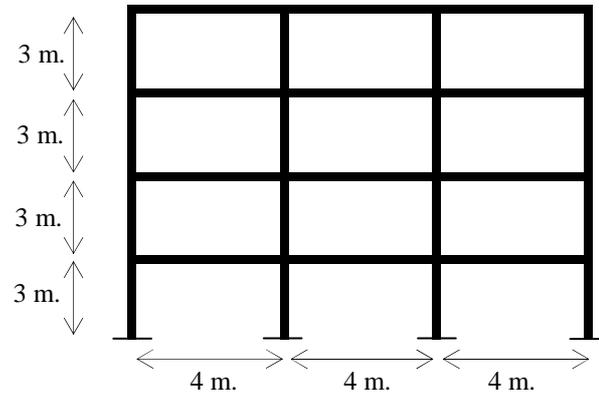
**Figure 5.** 4-storey RC frame used to verify the damage spectra
