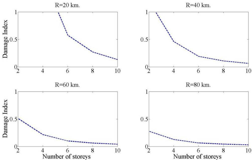
**Figure 7.** Variation of damage indices with building height for L'Aquila earthquake  $\mu=2$  and  $F_y/W=0.05$
