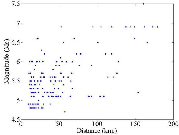
**Figure 2.** Distribution of the magnitude and distance of the ground motion records on soft soil
