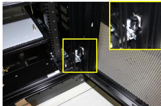
(b) Damage of the door hinge (After-shock 330%)
