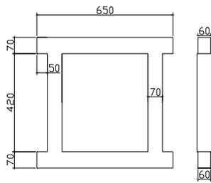
Figure 3.1. Dimension of the frame
