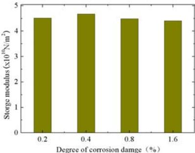
**Figure 2.7.** Influence of steel-bar corrosion on storage modulus
