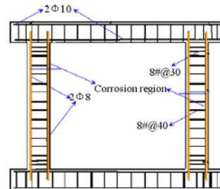
Figure 3.2 Reinforcement arrangement and corrosion region
