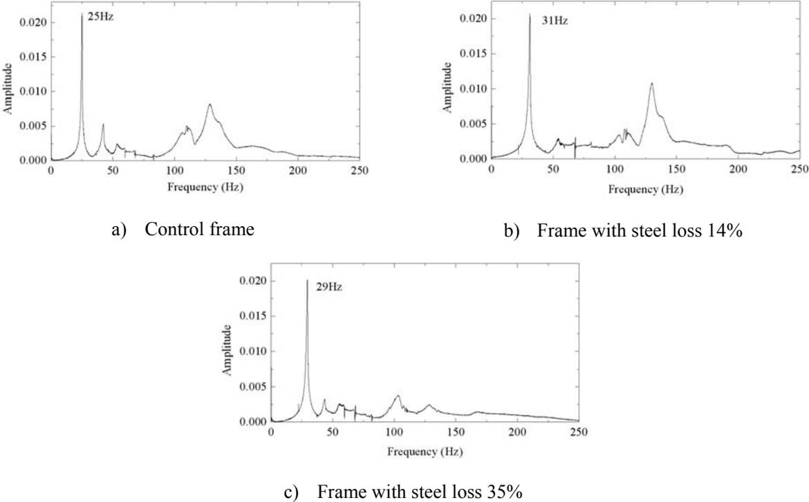
Figure 3.5. Fourier spectrum of accelerometer
