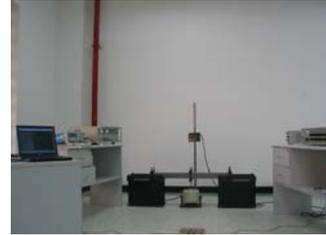
**Figure 2.3.** Three-point dynamic bending testing device
