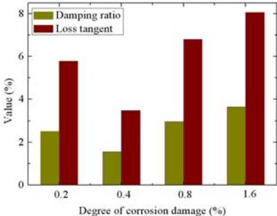
**Figure 2.6.** Influence of steel-bar corrosion on damping ratio and loss tangent
