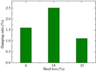
Figure 3.6. The influence of steel corrosion on damping ratio of frame
