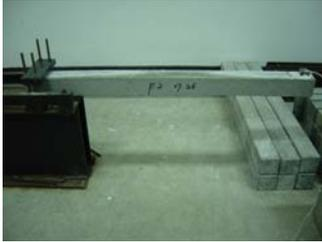
**Figure 2.2** Cantilever device for damping test
