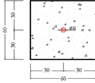
**Figure 2.1.** Reinforcement arrangement of beams
