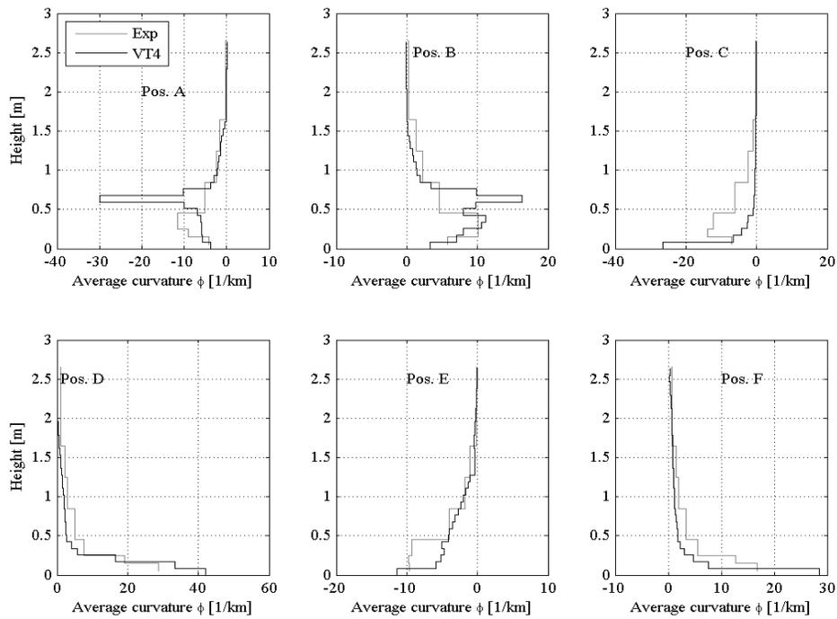
**Figure 4.3.** Comparison of the results obtained from VecTor4 with the experimental results during the  $\mu_{\Delta}=3.0$  cycles at Positions A, B, C, D, E and F: curvatures numerically determined from the nodal displacements of the mesh elements (VT4) compared with curvatures experimentally determined from LVDT measurements.
