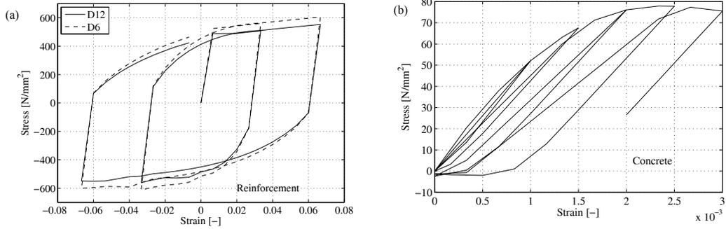
**Figure 3.2.** Material models: (a) reinforcement model and (b) concrete model: unconfined concrete in cyclic compression.
