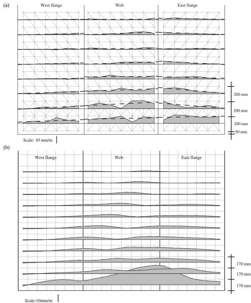
**Figure 4.2.** Comparison of the results obtained from VecTor4 with the experimental results at Position E during the  $\mu_{\Delta} = 3.0$  cycles (at Position E the west flange end is in compression): (a) vertical strain profile of the wall experimentally determined from Demec measurements and (b) vertical strain profile of the wall numerically determined.
