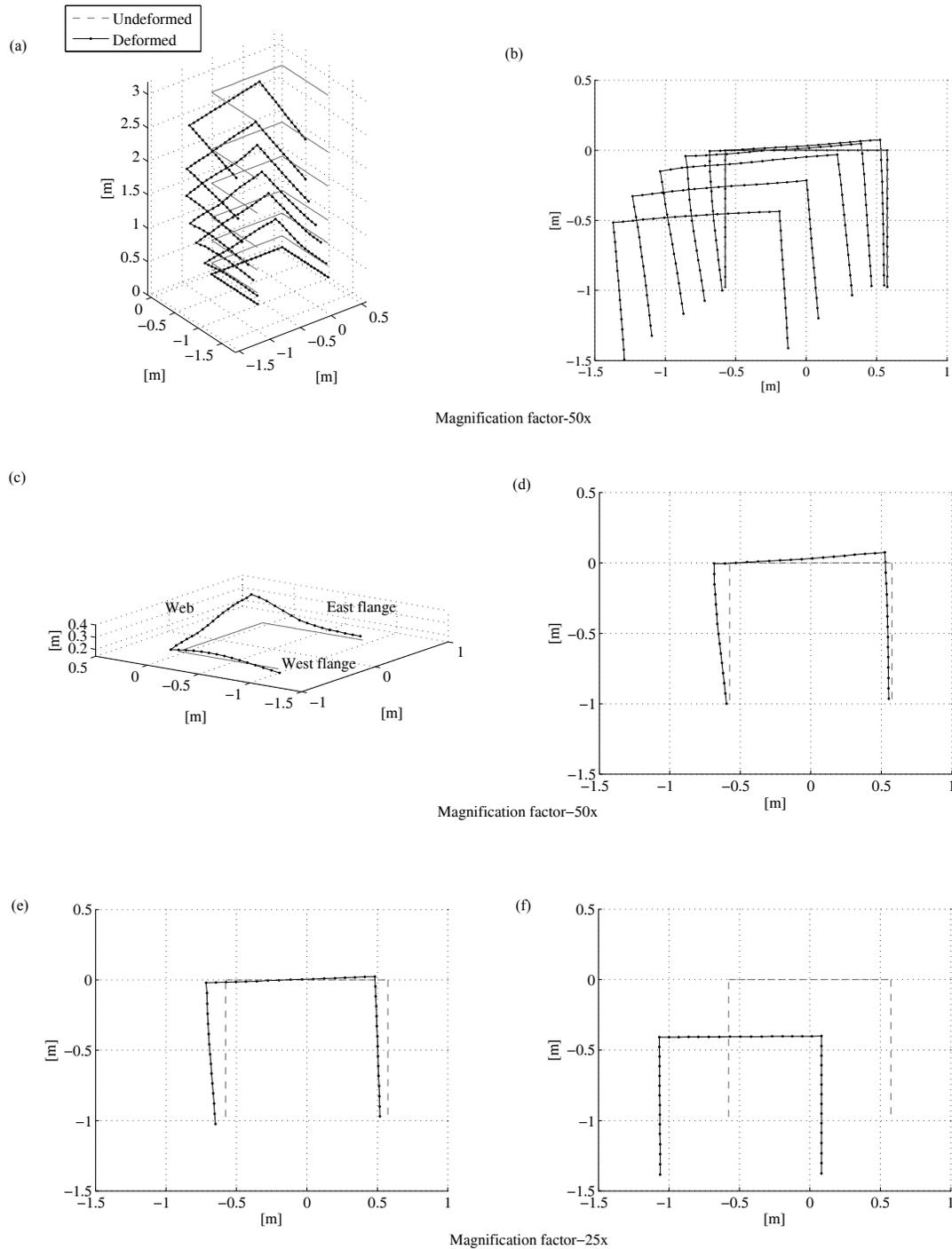
**Figure 5.3.** Numerically determined deformed shape of the wall at Position E at the peak of the  $\mu_{\Delta}=3$  cycle (at Position E the west flange end is in compression): (a) 3D deformed shape, (b) 3D deformed shape – view from the top, (c) 3D deformed shape of the element nodes for CS0.06, (d) CS0.06, (e) CS0.2 and (f) CS1. The displacements were magnified by factors of 50 or 25 as indicated below the subfigures.
