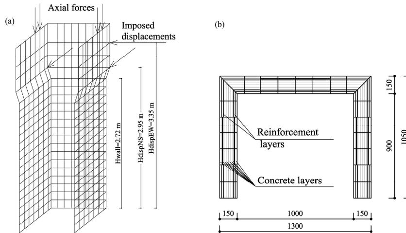
**Figure 3.1.** Geometry of the shell element model: (a) 3D mid-surface of the mesh and points of load application and (b) cross-section mesh. All dimensions are in *mm* unless otherwise specified in the figure.
