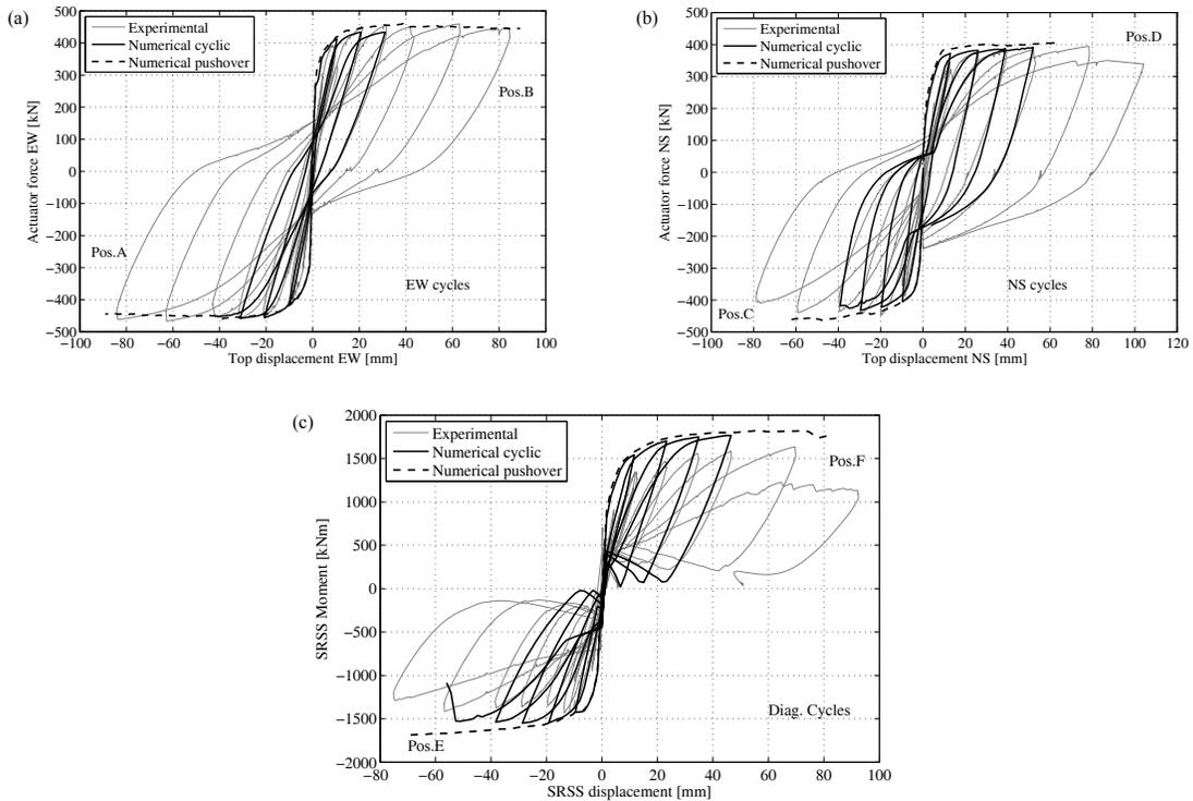
**Figure 4.1.** Comparison of the results obtained from VecTor4 with the experimental results: Force-displacement hysteresses for cycles in the EW and the NS directions (a-b). Moment-displacement hysteresses for the diagonal direction (c). Pushover analyses results are also included (a-c).
