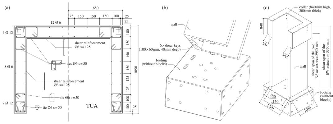
**Figure 2.2.** TUA geometry: (a) Cross-section, (b) shear keys and (c) elevation (taken from Beyer *et al.* [2008a]). All dimensions are in *mm*.
