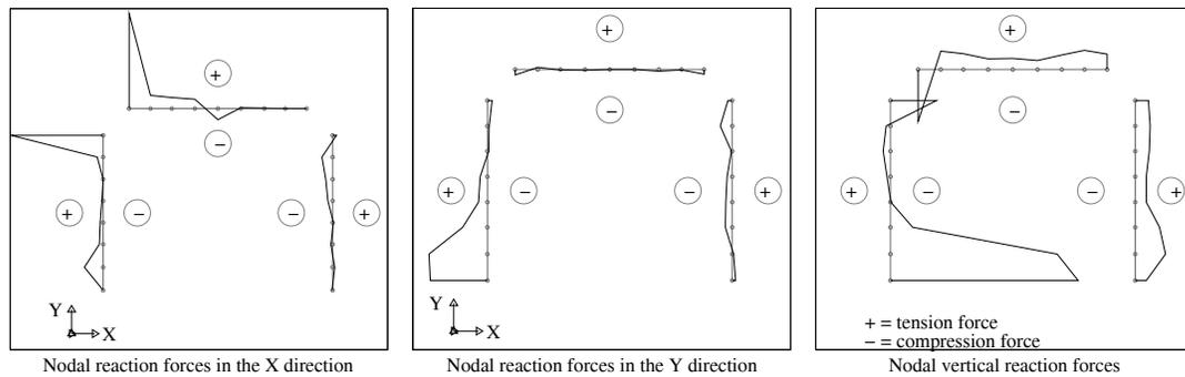
**Figure 5.1.** Numerically determined qualitative distribution of reaction forces at the base of the wall at Position E at the peak of the  $\mu_{\Delta}=3$  cycle (at Position E the west flange end is in compression).
