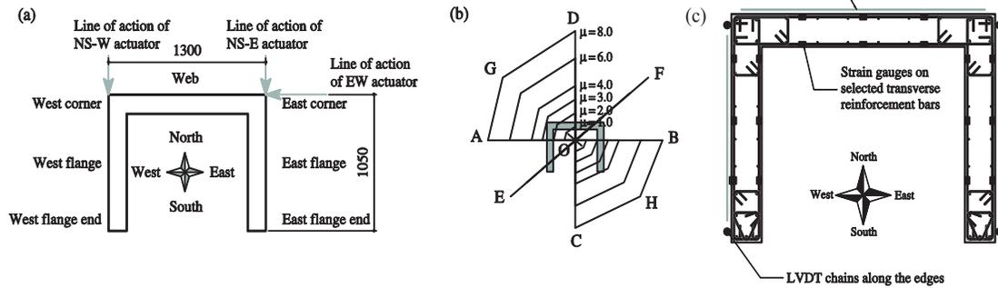
**Figure 2.1.** (a) Labelling of different wall sections and lines of action of the actuators, (b) bi-directional displacement loading history and (c) wall instrumentation (taken from Beyer *et al.* [2008a]). All dimensions are in *mm*.
