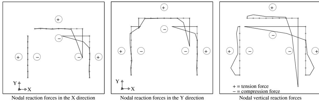
**Figure 5.2.** Numerically determined qualitative distribution of reaction forces at the base of the wall at Position F at the peak of the  $\mu_{\Delta}=3$  cycle (at Position F the corner of the web and of the east flange is in compression).
