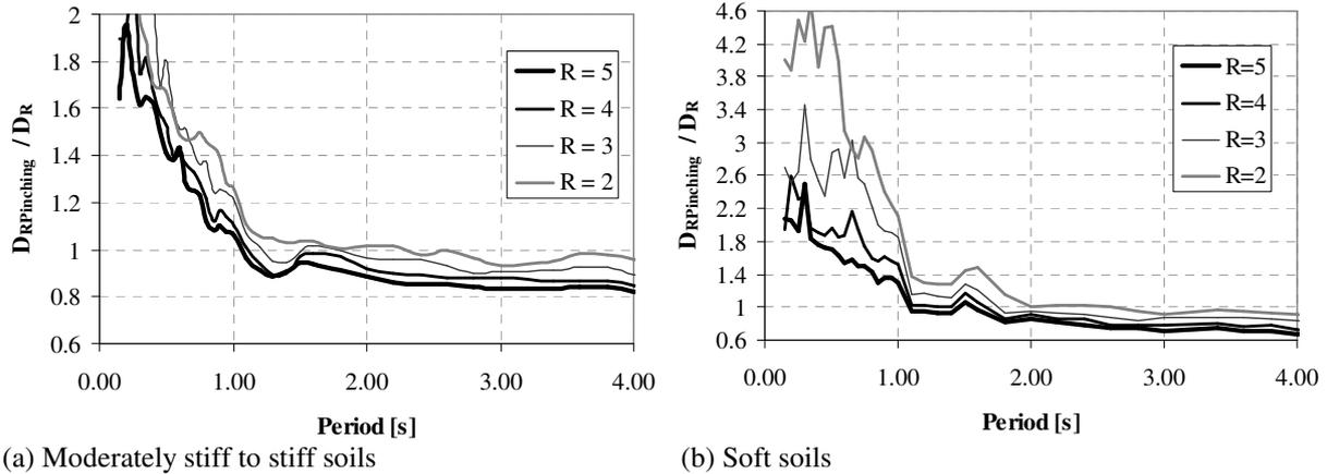
**Figure 7.** Mean Park and Ang Damage Index of pinching systems with  $P = 0.3$  normalized by mean Park and Ang Damage index of bi-linear models
