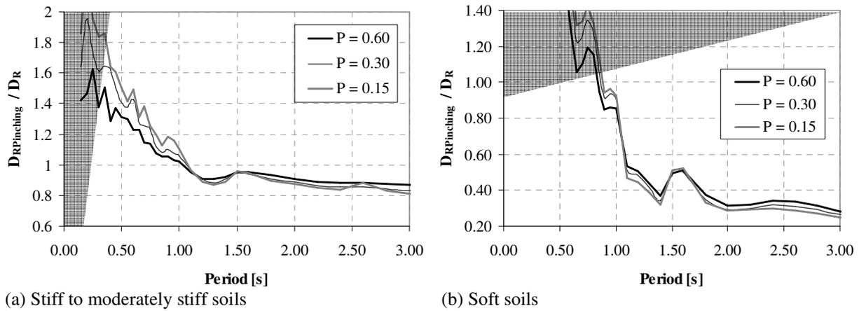
**Figure 8.** Mean Park and Ang Damage Index of pinching systems normalized by mean Park and Ang Damage index of bi-linear models for  $R = 5$
