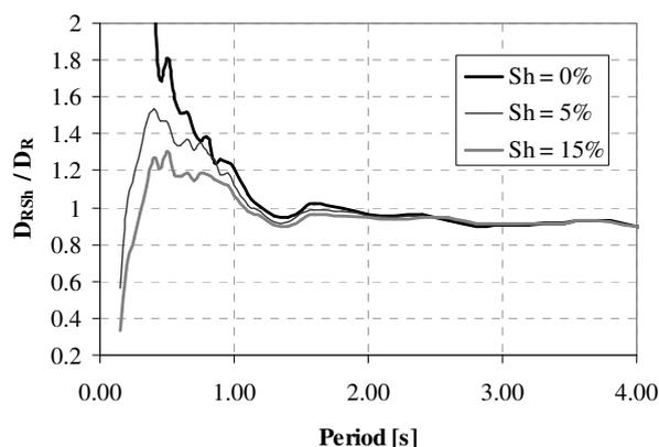
**Figure 9.** Mean Park and Ang Damage Indexes for pinching structures normalized by mean Park and Ang Damage Indexes in bi-linear systems for different strain hardening coefficients  $R = 5$ .
