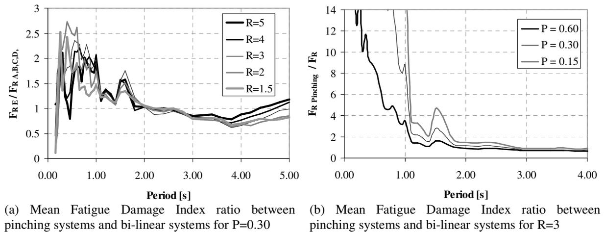
**Figure 5.** Fatigue Damage Index ratios for soft soils
