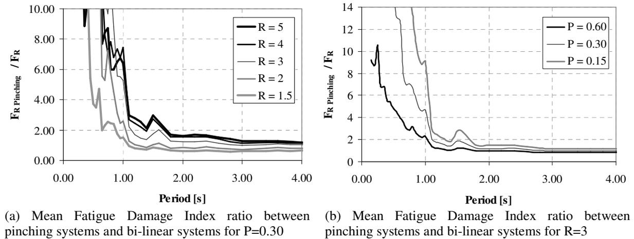
**Figure 4.** Fatigue Damage Index ratios for moderately stiff to stiff soils
