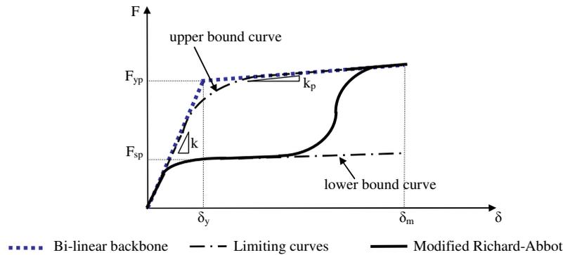
**Figure 1.** Bi-linear and modified Richard-Abbott force-deformation relationships
