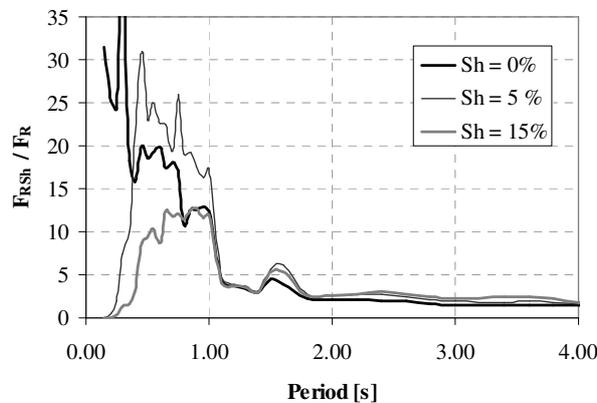
**Figure 9.** Mean Fatigue Damage Indexes for pinching structures normalized by mean Fatigue Damage Indexes in bi-linear systems for different strain hardening coefficients  $R = 5$ .
