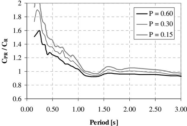
**Figure 3.** Mean inelastic displacement ratios of pinching systems normalized by mean displacement ratios of bi-linear systems. Average for all strength values on moderately stiff to stiff soils as a function of pinching factor ( $P$ )
