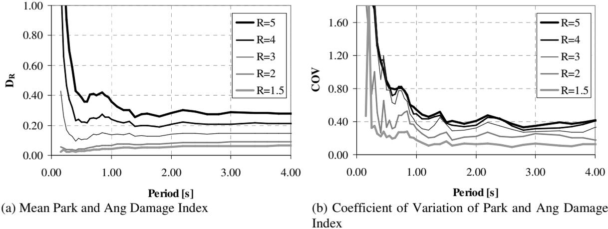
**Figure 6.** Park and Ang Damage Index of bi-linear systems on stiff to moderately stiff soils
