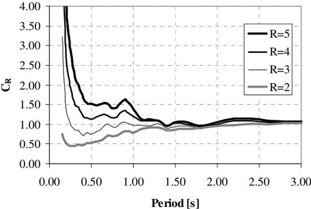
**Figure 2.** Mean inelastic displacement ratios for moderately stiff to stiff soil ground-motions on bi-linear systems
