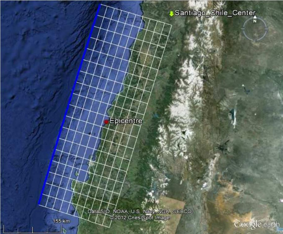
**Figure 2.4.** 2010 Chile earthquake rupture location adopted for the simulations.
