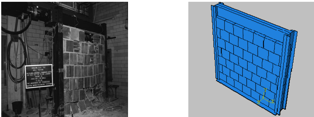
Figure 1. schematic view of test specimen and Finite element model of infilled steel frame
