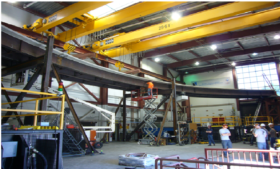
Figure 2. Bridge Model Assembled in Large-Scale Structures Laboratory
