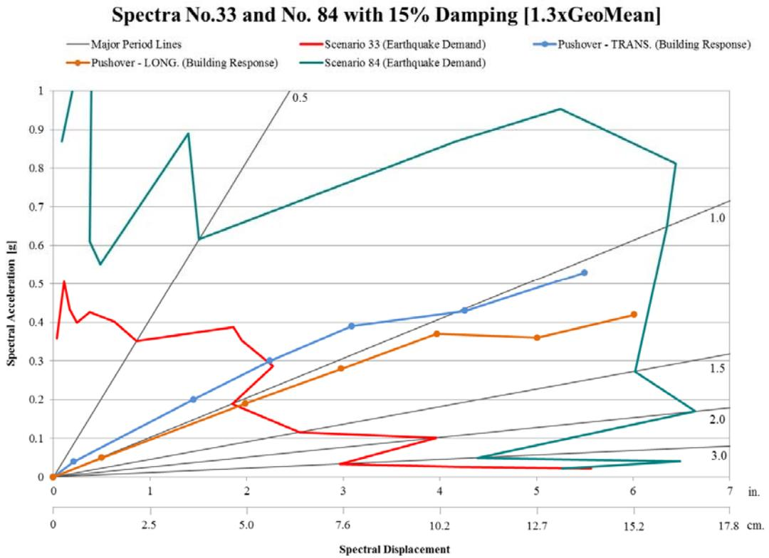
**Figure 4.** ADRS plot of unidirectional pushover curves and scenario earthquake spectra.
