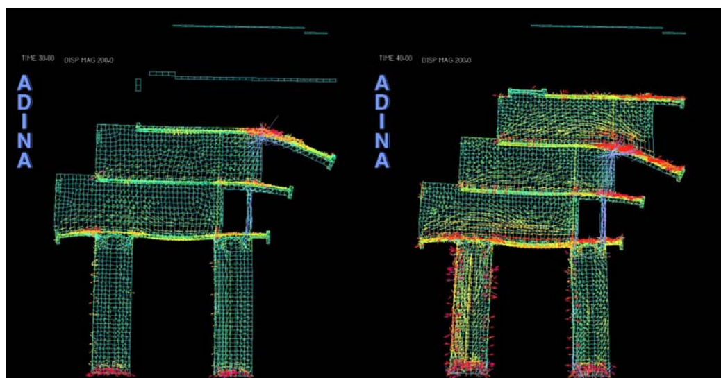
Figure 6. Principal tensile vector plot. Construction sequence to 6th floor (left) and to the 7th floor (right)
