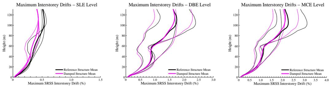
Figure 9.1 Maximum Interstorey Drifts – East-West Direction
