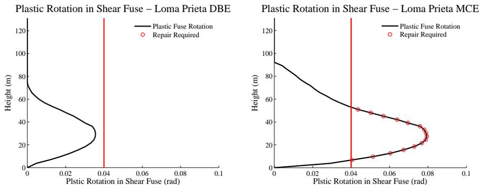
**Figure 9.8** Peak Shear Fuse Plastic Rotations – Loma Prieta
