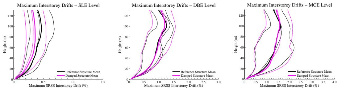
Figure 9.2 Maximum Interstorey Drifts – North-South Direction
