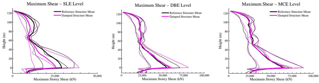
**Figure 9.3** Maximum Storey Shear – East-West Direction
