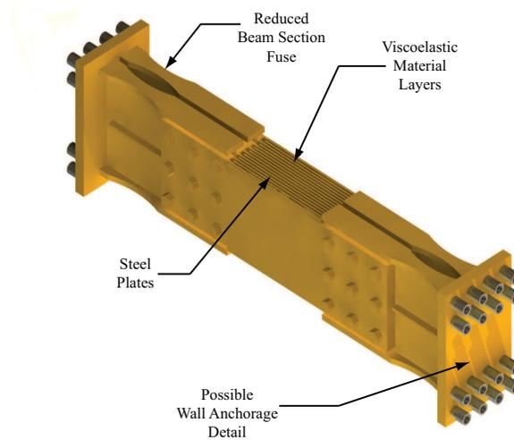
**Figure 2.1** Viscoelastic Coupling Damper (VCD)
