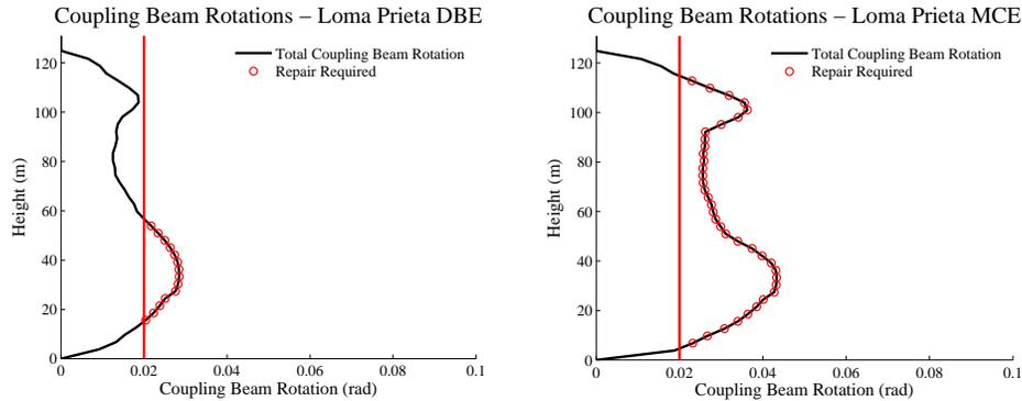
**Figure 9.7** Peak Coupling Beam Rotations – Loma Prieta
