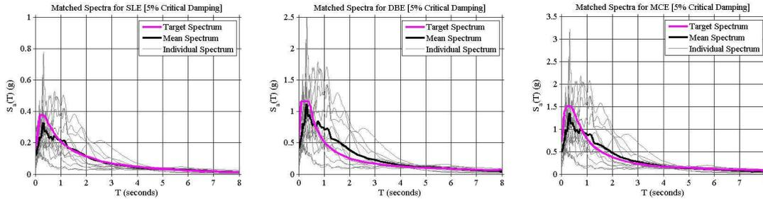
**Figure 6.1** Scaled site specific spectra
