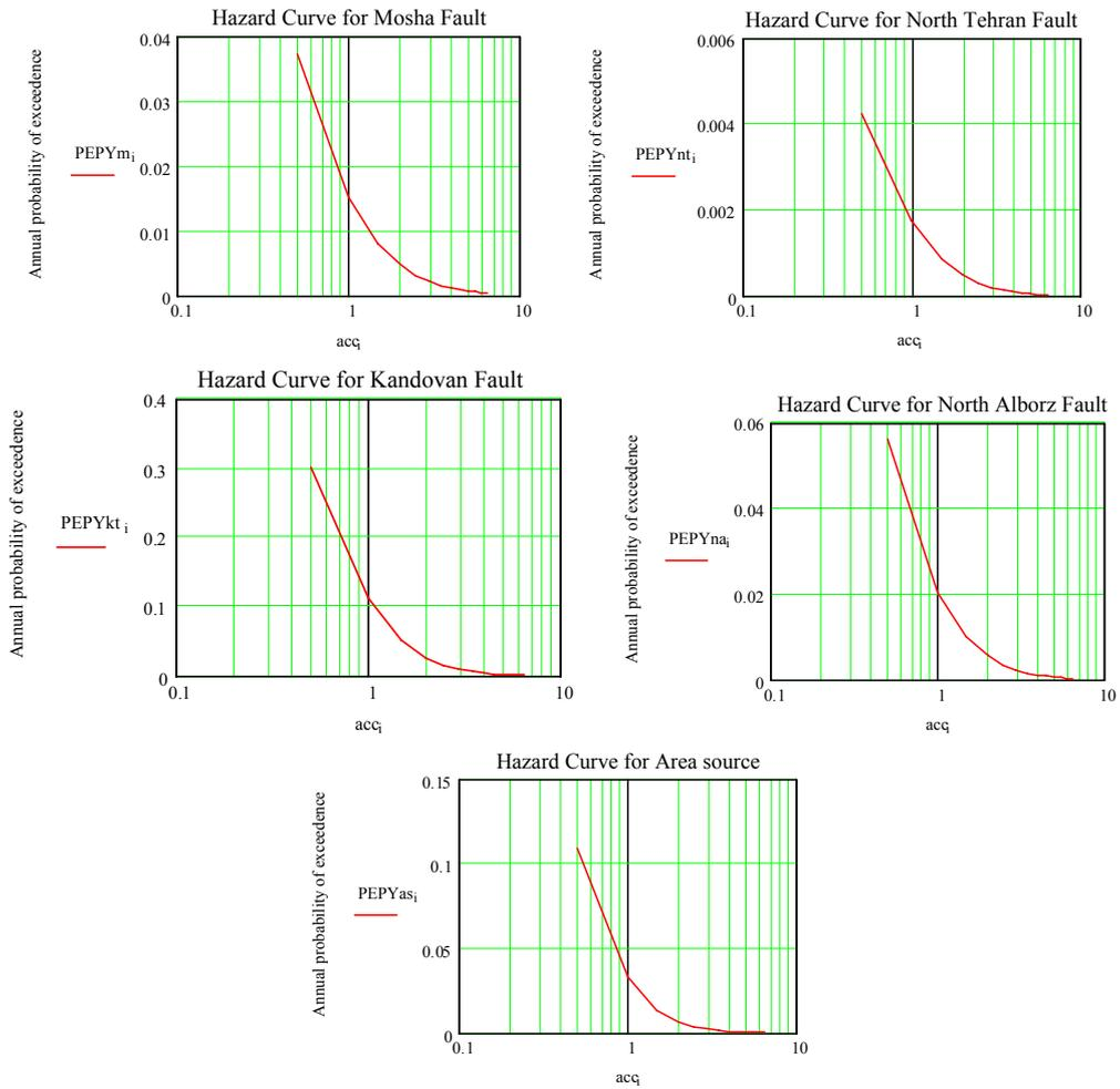
**Figure 2.** The hazard curve obtained for the seismic sources by Zare-Ashtiany attenuation relationship (H Component)
