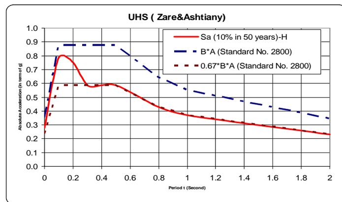
**Figure 6.** Comparison among UHS curves for different probability of exceedence and Iranian Seismic Code design spectrum (Standard No. 2800-05) for Life Safety Level
