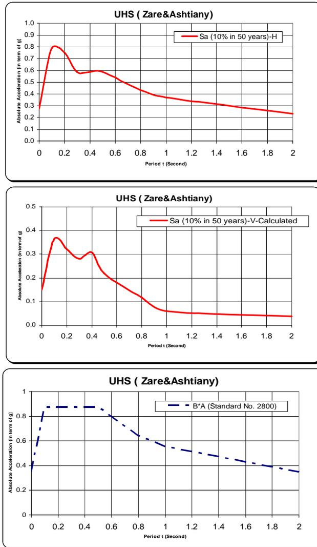
**Figure 5.** UHS curves for 10% probability of exceedence in 50 years (H & V Comp.) and Iranian Seismic Code design spectrum (Standard No. 2800-05) for Life Safety Level
