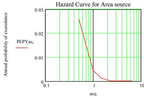
**Figure 3.** The hazard curve obtained for the seismic sources by Zare-Ashtiany attenuation relationship (V Component)
