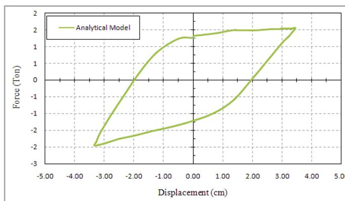
**Figure 3.4.** Last Hysteresis Loop of Analytical Model in Single-layer Specimen
