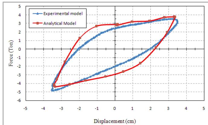
**Figure 3.9.** Analytical and Experimental Hysteresis Loops of the Two-layer Model
