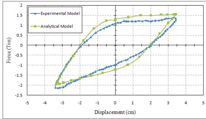
**Figure 3.5.** Analytical and Experimental Hysteresis Loops of Single-layer Specimen
