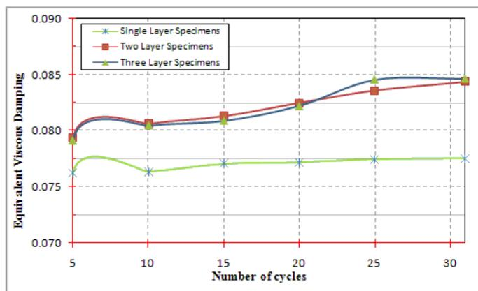
**Figure 4.5.** Equivalent Viscous Damping Level Curve in Single-layer, Two-layer and Three-layer Models
