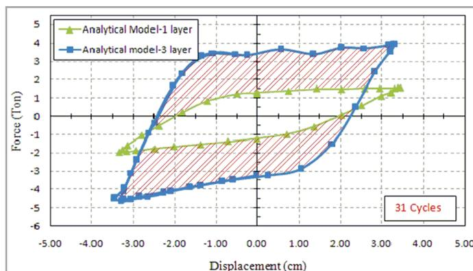
**Figure 4.2.** Comparison of the Hysteresis Loop of Single-layer and Three-layer Specimens
