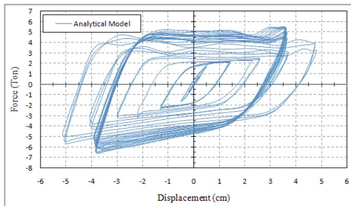
**Figure 3.10.** Hysteresis Loops of Three-layer Analytical Model
