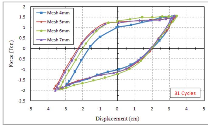
**Figure 3.2.** Hysteresis Loops Related to Single-layer Tube with Different Meshing Sizes
