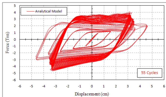
**Figure 3.7.** Hysteresis Loops of the Analytical Model in Two-layer Model
