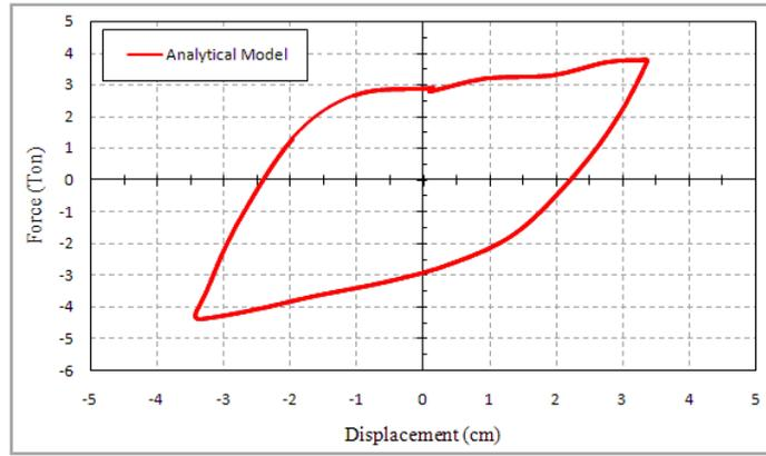
**Figure 3.8.** Last Hysteresis Loop of the Analytical Model in Two-layer Model
