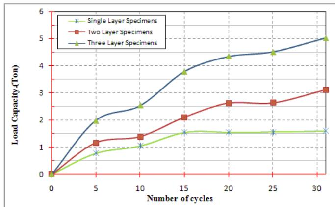
**Figure 4.4.** Plastic Capacity Level Curve in Single-layer, Two-layer and Three-layer Models
