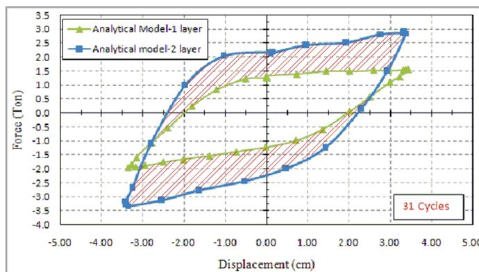
**Figure 4.1.** Comparison of the Hysteresis Loop of Single-layer and Two-layer Specimens
