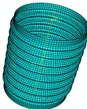
**Figure 3.1.** Single Layer Analytical Model Based on Finite Element Method
