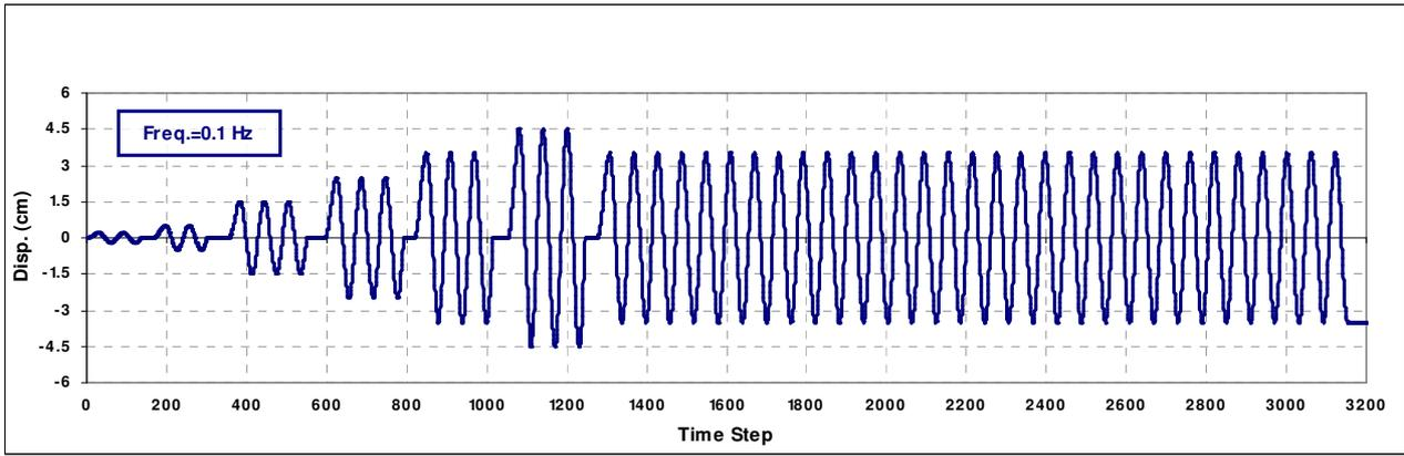
**Figure 2.2.** Axial Cyclic Loading Regime Applied to Experimental Specimens
