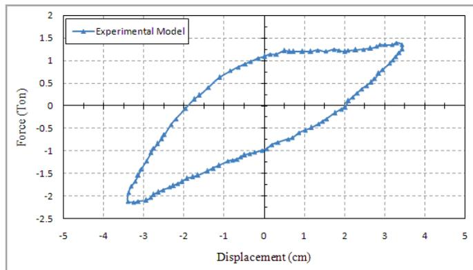
**Figure 2.3.** Last Hysteretic Loops of Single Layer Specimen
