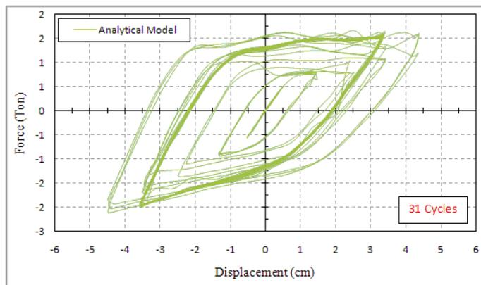
**Figure 3.3.** Hysteresis Loops of the Analytical Model in Single-layer Specimen
