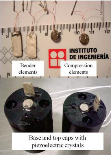
Figure1. Piezoelectric crystals for generating and recording seismic waves
