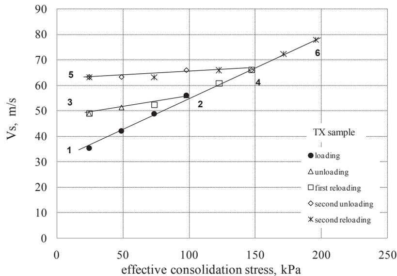
**Figure 9.** Shear wave velocities in the TX sample as a function of effective consolidation stress
