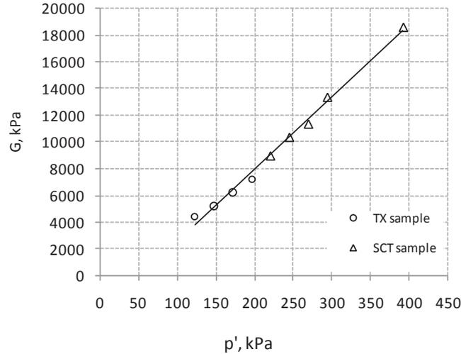
**Figure 12.** Shear moduli as a function of  $p'$  for normally consolidated states, both samples.
