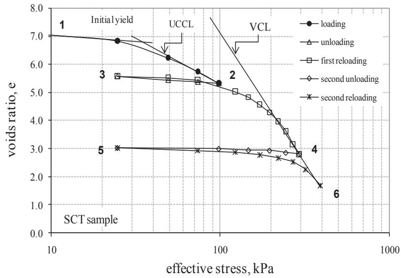
**Figure 6.** Isotropic compressibility curve for the reconstituted SCT sample.
