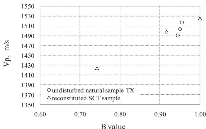
**Figure 3.** Values of compression wave velocities plotted against Skempton's B parameter during saturation.
