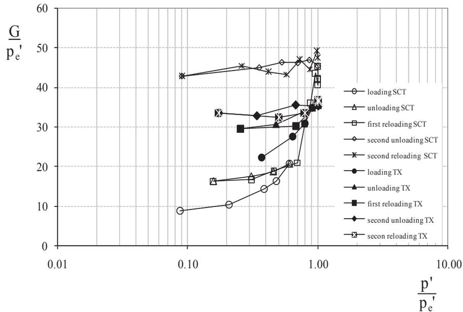
**Figure 11.** Normalized shear moduli plotted against  $p'/p'_e$  for samples TX and SCT
