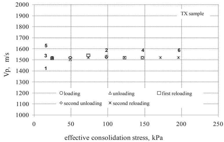
**Figure 7.** Compression wave velocities measured during isotropic loading of the natural TX sample.
