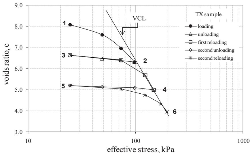
Figure 5. Isotropic compressibility curve for the TX natural sample.
