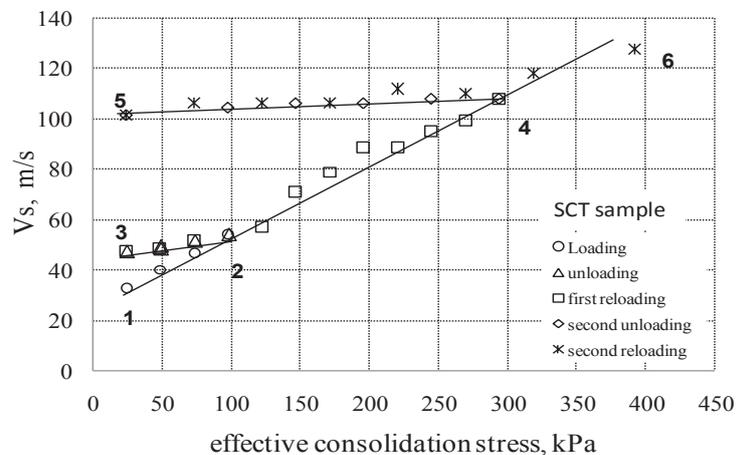
**Figure 10.** Shear wave velocities in the SCT sample as a function of effective consolidation stress
