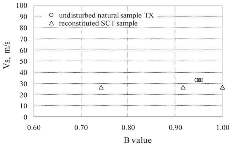
Figure 4. Values of shear wave velocities plotted against Skempton's B parameter during saturation.
