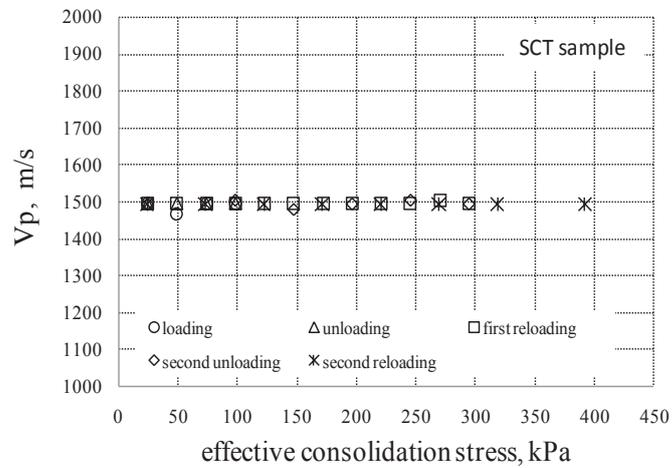
**Figure 8.** Compression wave velocities measured during isotropic loading of the reconstituted SCT sample.
