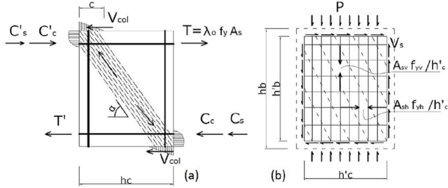
**Figure 1.** (a) Strut Mechanism; (b) Truss Mechanism; (according to the Model of Paulay and Priestley, 1992)
