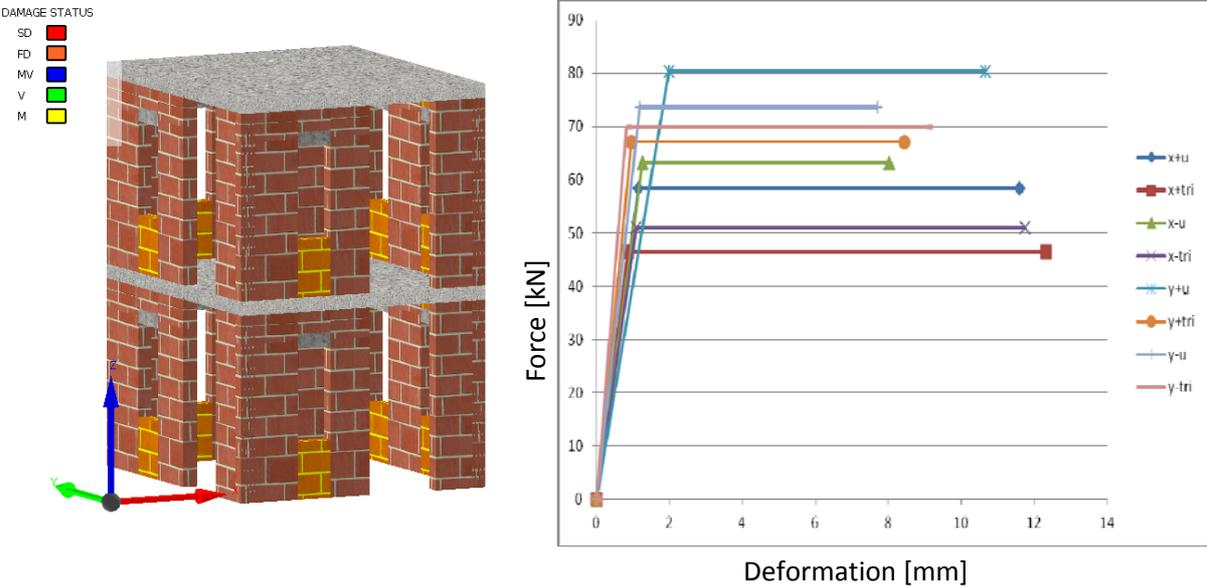
**Figure 8.** Numerical modelling results of model II: 3-D sketch model and linearized pushover curves for deformations in positive/negative x/y-direction using uniform or triangular displacement
