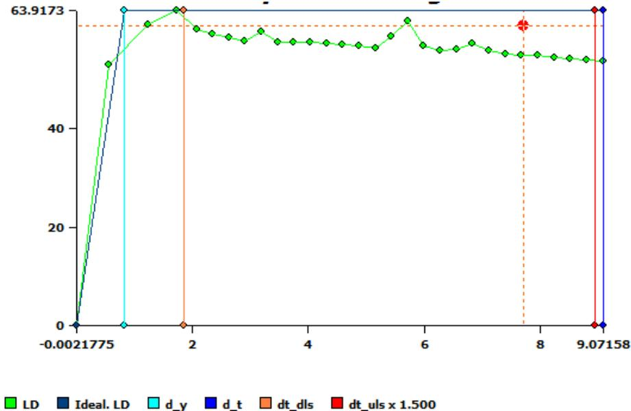
**Figure 6.** Typical pushover curve showing numerical results (green line), linearized pushover curve (blue line), and target limit states according to Eurocode 8 with deformation limit state (orange line) and ultimate limit state (red solid line)
