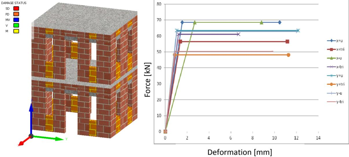
**Figure 7.** Numerical modelling results of model I: 3-D sketch model and linearized pushover curves for deformations in positive/negative x/y-direction using uniform or triangular displacement
