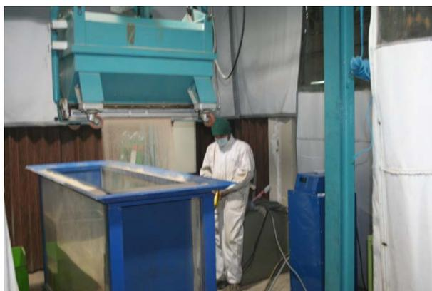
**Figure 4.** The pluviation technique with an electric sand rainer
