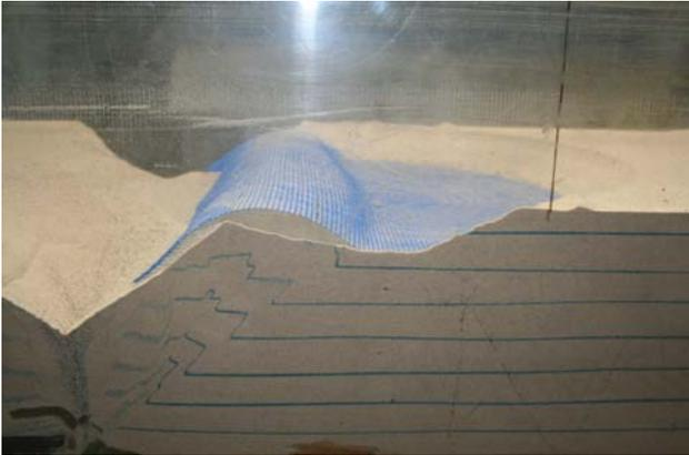
**Figure 8.** Geogrid situation beneath foundation after test 23N
