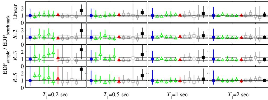
(a) Plan B - EDP: Displacement. - Direction:  $x$  - Point: Center of mass.
