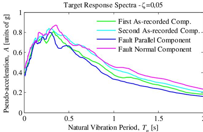
**Figure 4.3.** Geometric-mean pseudo-acceleration response spectra of 30 unscaled records.
