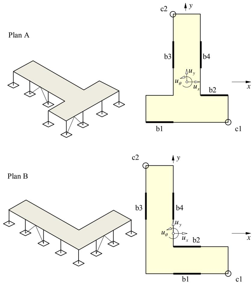
**Figure 5.1.** Schematic isometric and plan views of the selected structural systems with degrees of freedom noted; buckling-restrained braced frames are highlighted.
