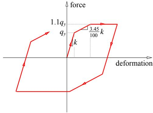
**Figure 5.2.** Constitutive model used for the buckling-restrained braces (BRBs).
