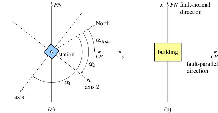
**Figure 4.2.** (a) Reference axes for the fault and the instrument with relevant angles noted. (b) Reference axis for the building.
