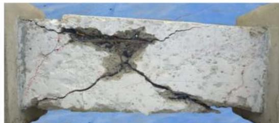
Figure (10-b) Failure Mode .E15
