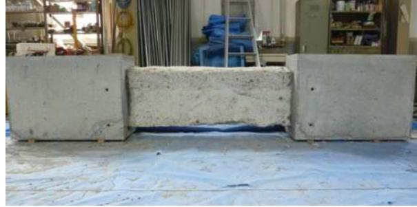
Figure 4. Completed specimen with stubs
