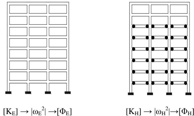
**Figure 3.** Dynamic properties of the elastic and hardening stages of behaviour
