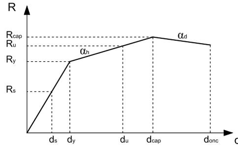
**Figure 4.** Design behaviour curve
