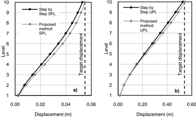
Figure 5. Comparison of displacements: a) service; b) ultimate
