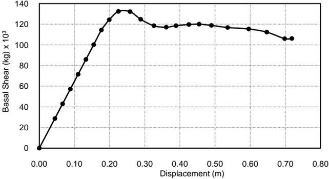
Figure 7. Capacity curve obtained from Incremental Dynamic Analysis
