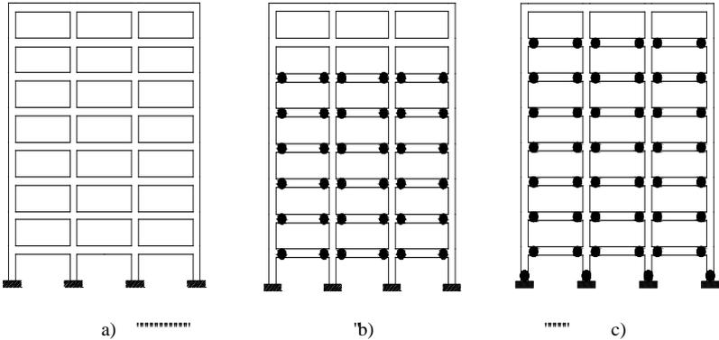
**Figure 2.** Damage distributions associated to the three stages of behaviour: a) elastic; b) hardening; c) degrading
