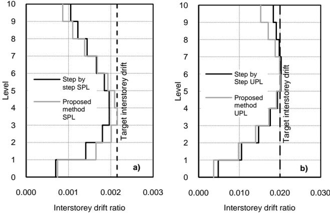
Figure 6. Comparison of interstorey drifts: a) service; b) ultimate
