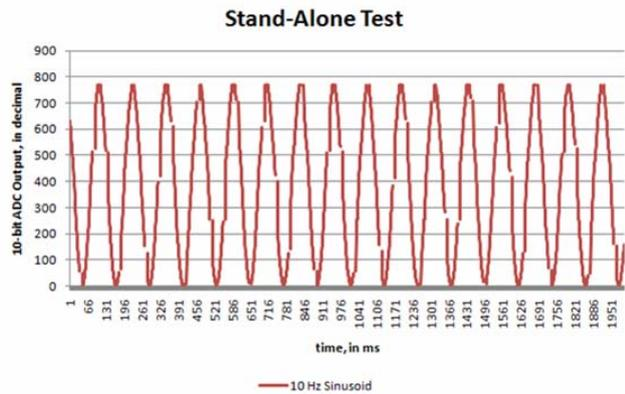
Figure 6. Reconstructed Waveform from the Sampling Test
