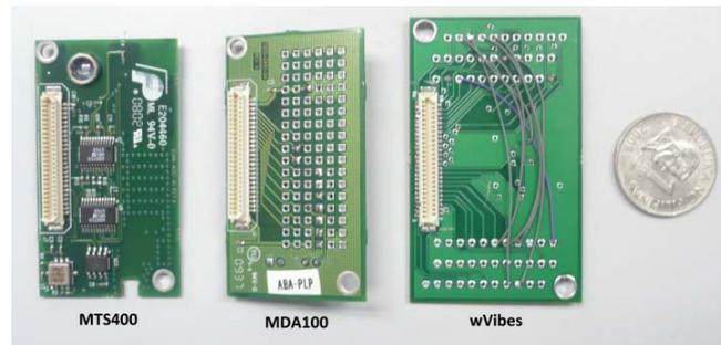
**Figure 3.** Sensor Node with other Commercially Available Sensor Boards
