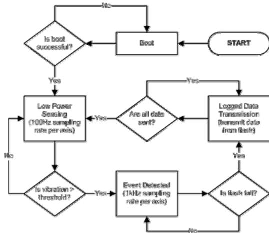
Figure 5. Slave Node Operation Diagram
