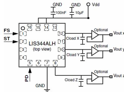
**Figure 4.** LIS344ALH signal conditioning
