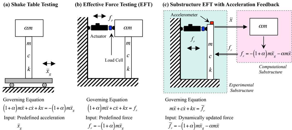
**Figure 1.** Schematics of various experimental methods: (a) shake table test; (b) effective force test; and (c) substructure effective force test.
