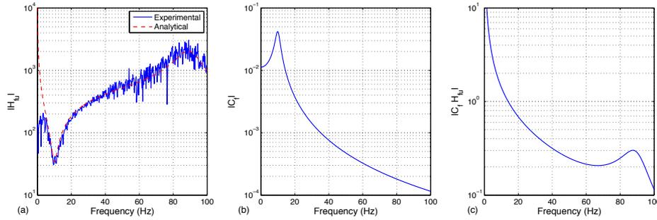
**Figure 3.** Open-loop transfer functions: (a) transfer function from valve voltage to actuator force; (b) controller transfer function; and (c) loop transfer function.
