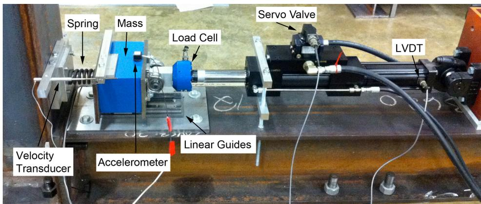
**Figure 2.** The mass-spring-actuator system for EFT at JHU.
