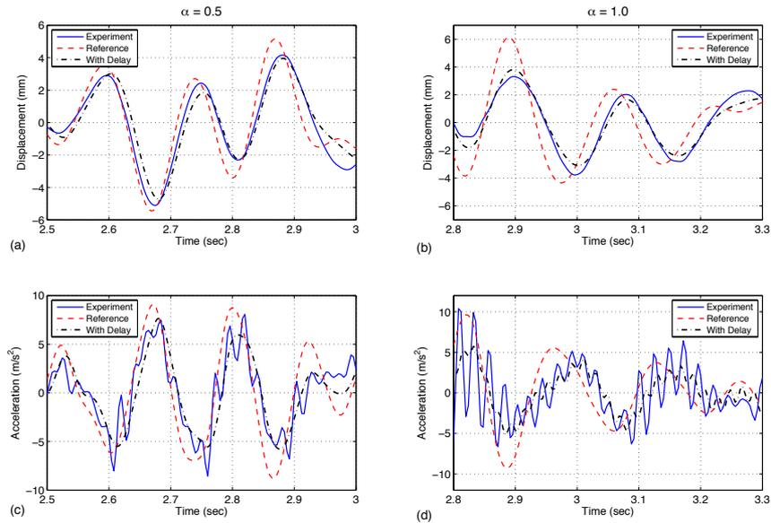
**Figure 7.** Comparison of time histories among reference, experiment and numerical simulations with actuator delay: (a) displacement at  $\alpha = 0.5$ ; (b) displacement at  $\alpha = 1.0$ ; (c) acceleration at  $\alpha = 0.5$ ; (d) acceleration at  $\alpha = 1.0$ .
