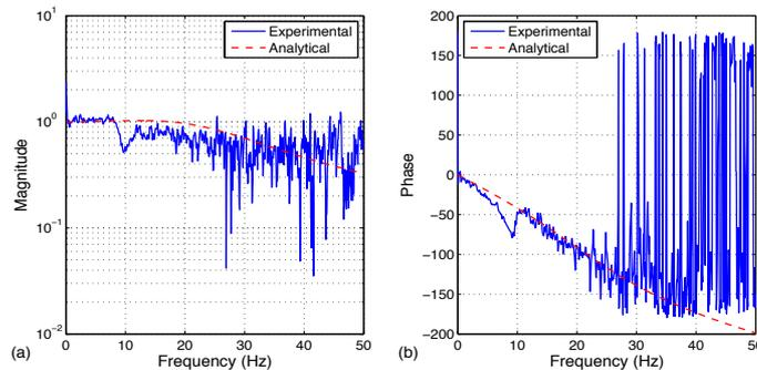
**Figure 4.** Closed-loop transfer function of actuator force: (a) magnitude and (b) phase.
