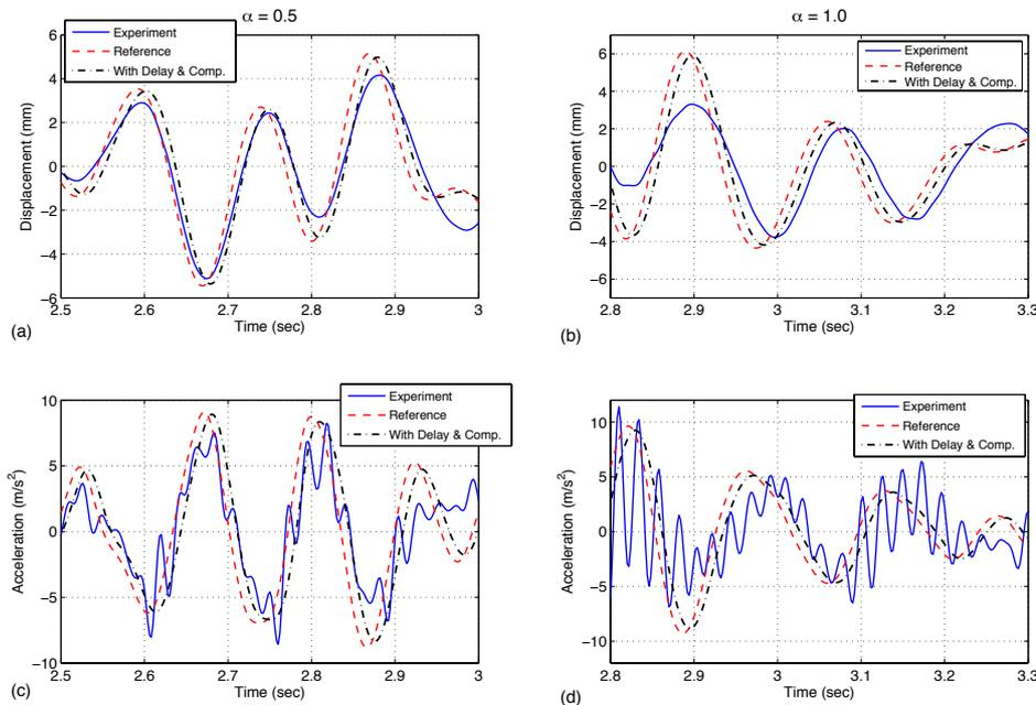
**Figure 7.** Comparison of time histories among reference, experiment and numerical simulations with delay compensation: (a) displacement at  $\alpha = 0.5$ ; (b) displacement at  $\alpha = 1.0$ ; (c) acceleration at  $\alpha = 0.5$ ; (d) acceleration at  $\alpha = 1.0$ .
