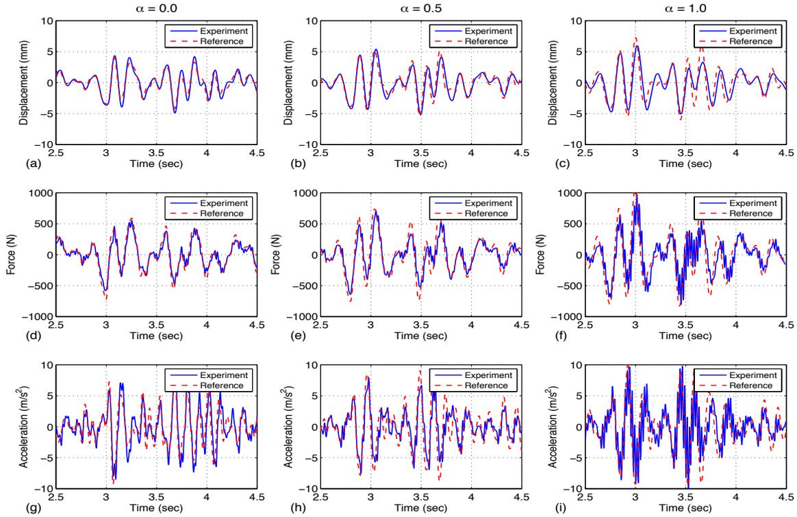
**Figure 6.** Time histories under the 1995 Kobe earthquake; (a), (b), and (c) displacement time histories for  $\alpha = 0$ , 0.5 and 1.0, respectively; (d), (e), and (f) force time histories for  $\alpha = 0$ , 0.5 and 1.0, respectively; and (g), (h), and (i) acceleration time histories for  $\alpha = 0$ , 0.5 and 1.0, respectively.
