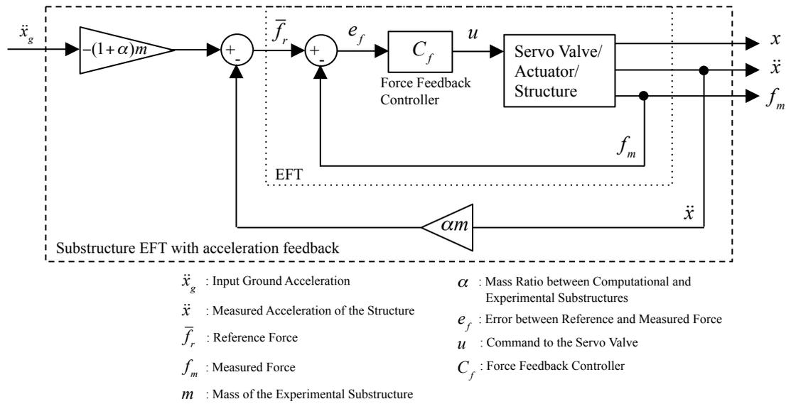
**Figure 5.** A block diagram of the substructure effective force test method incorporating acceleration feedback for simulated inertial force.
