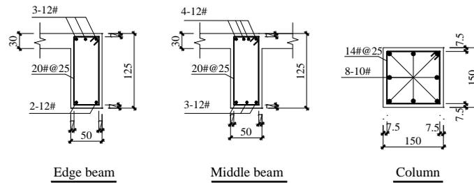
Figure 7 Rebar details of different cross sections
