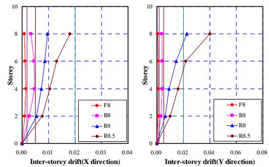
Figure 28 The inter-story drift of TRC prototype
