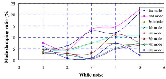
Figure 18 The changing of mode damping ratio of semi-recycled concrete frame model
