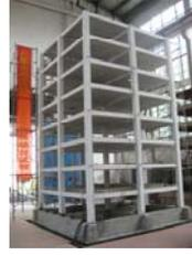
**Figure 6** The panorama of totally-recycled concrete model
