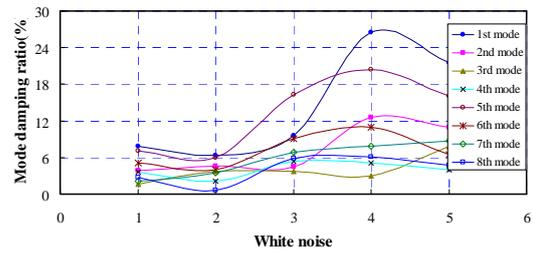
Figure 20 The changes of damping ratio of totally-recycled concrete frame model
