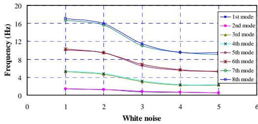
Figure 19 The changes of frequencies of totally-recycled concrete frame model
