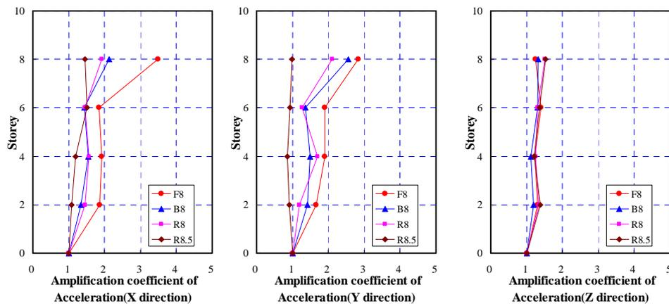
Figure 21 The amplification coefficient of acceleration at different levels of intensity of degree (SRC)
