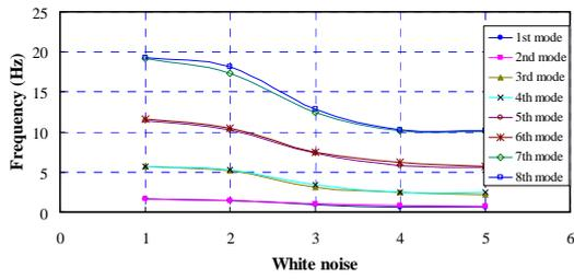
Figure 17 The changing of mode frequencies of semi-recycled concrete frame model
