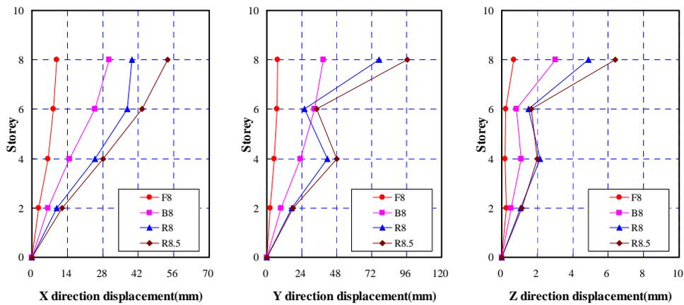
Figure 24 The storey displacement envelope at different level of intensity (TRC)
