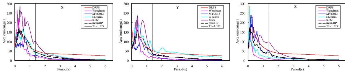
Figure 8 The response spectra of input ground motions and designed response spectrum
