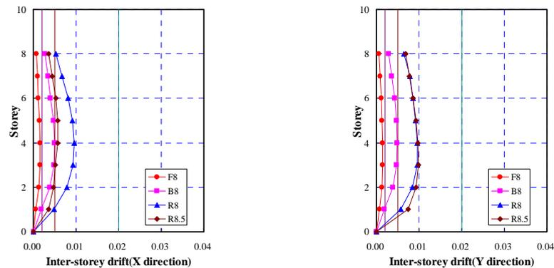
Figure 23 The calculation result of the inter-story drift of TRC prototype
