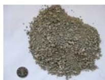
**Figure 3** Recycled coarse aggregate
