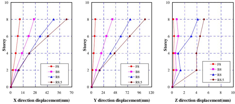
Figure 23 The storey displacement envelope at different levels of intensity (STRC)
