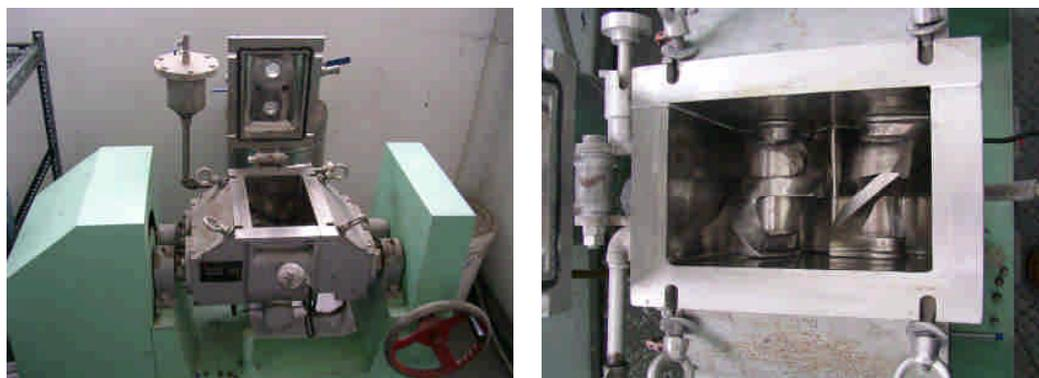
Figure 2.2. Blender for dispersion of STF fluid
