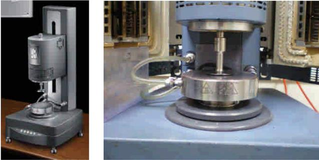
Figure 2.3. (a) Rheometer, (b) Cone and plate
