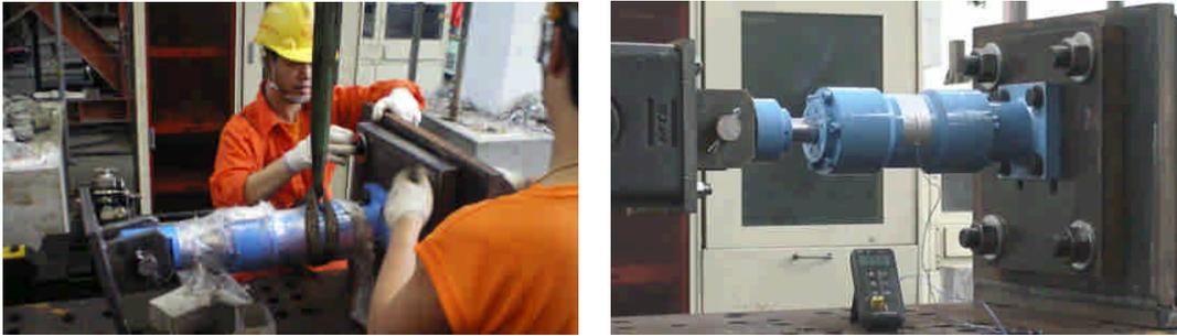
**Figure 4.1.** Layout of STF damper performance test
