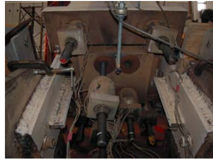
(b) Specimen 3 (towards 3% drift)
