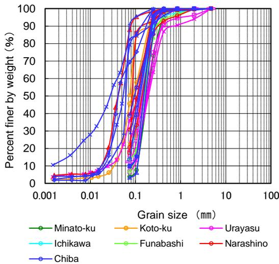
**Fig.3.1.** Grain size distribution curves of sand boiling in Tokyo Bay area
