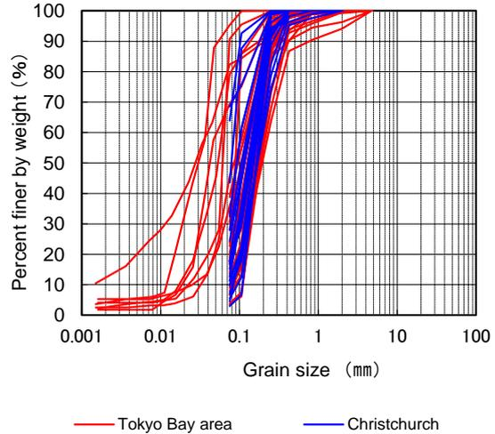
**Fig.3.2.** Grain size distribution curves of sand boiling in Tokyo Bay area and Christchurch
