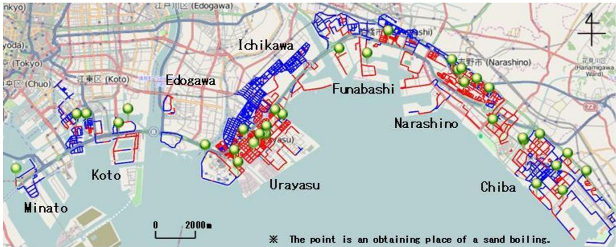
**Fig.2.1.** Liquefaction damage in Tokyo Bay area
