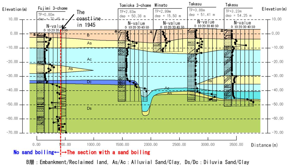
Fig.2.7. Estimated geological section of the Urayasu center section
