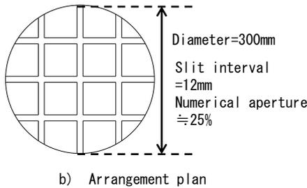
**Fig.4.1.** Schematic diagram of an experimental device
