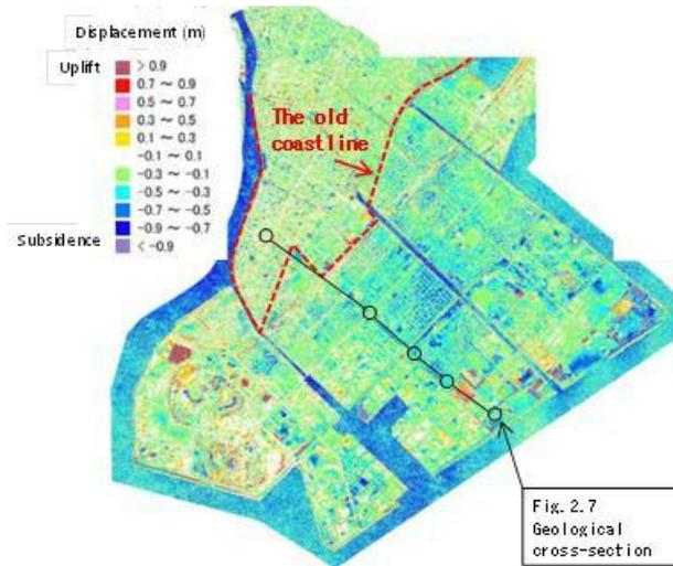
Fig.2.4. Displacement after the earthquake in Urayasu (Urayasu City, 2011)
