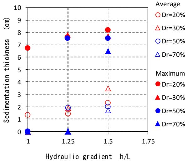
**Fig.4.4.** Relationship between hydraulic gradient and sedimentation thickness
