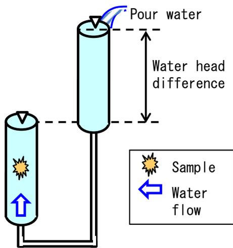
**Fig.5.1.** Experimental device to determine the ease of floating up of a soil particle
