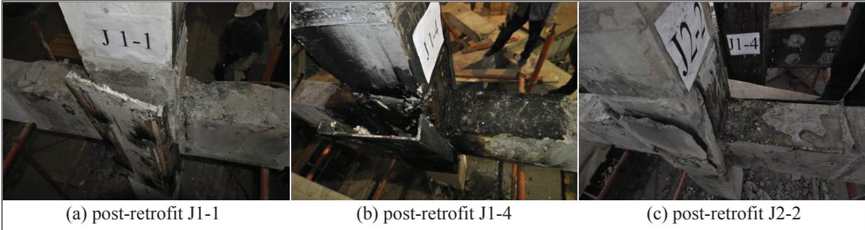
Figure 3.7. Damages of interface filler after cutting the enveloped steel jacket
