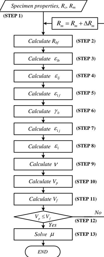
Figure 2. The calculation procedure
