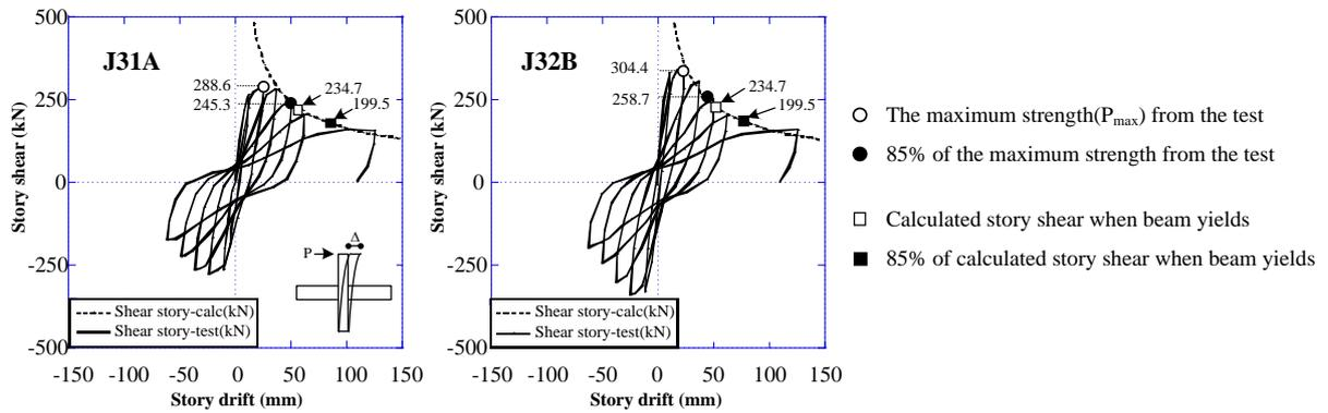
(b) Calculated curves compared with Kaku ' s test
