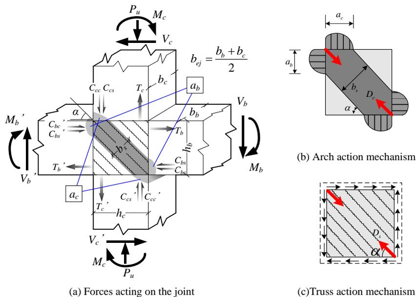
**Figure 5.** Two components to predict potential shear strength
