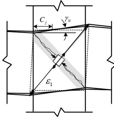
**Figure 4.** Increasing shear deformation
