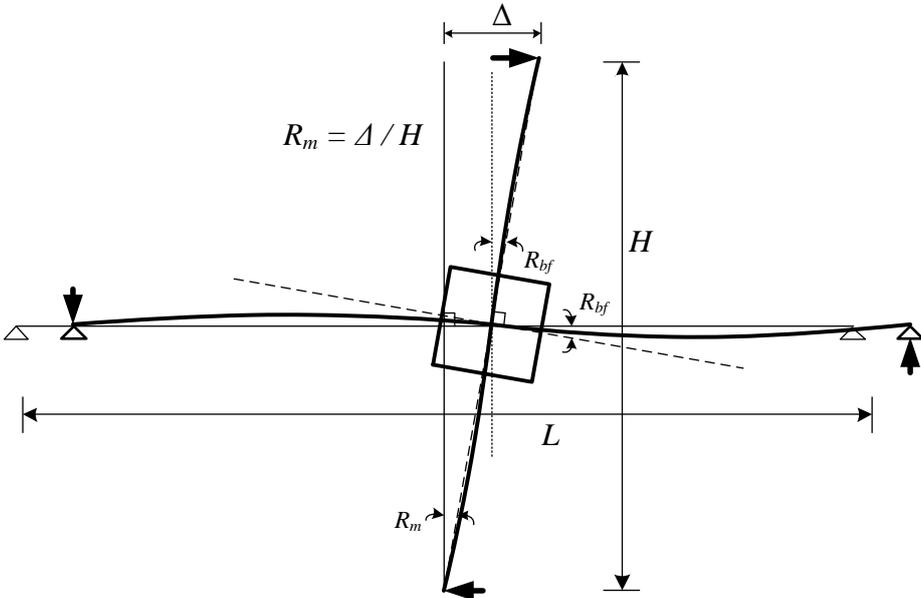
Figure 3. Joint deformation
