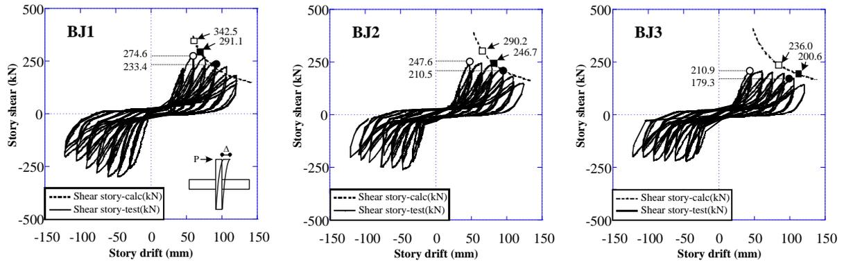
(a) Calculated curves compared with Lee ' s test
