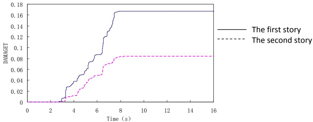
**Figure 7.** Comparison of average tensile damage parameter in the walls on the first floor and the second floor
