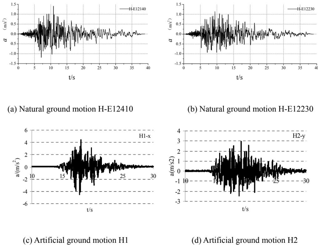
**Figure 4.** Acceleration waves
