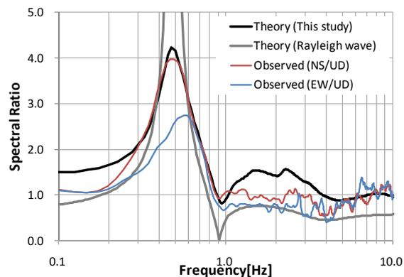
**Figure 3.2.** Theoretical H/V spectral ratio (black line) compared against H/V spectral ratio derived from ellipticity of Rayleigh waves (gray line) and observed H/V spectral ratio of June 21st, 2010 (red and blue lines)
