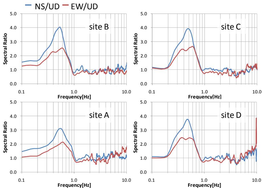
Figure 2.3. Average H/V spectral ratio of June 23<sup>rd</sup>, 2010, observed at sites A to D in Fig. 2.1b
