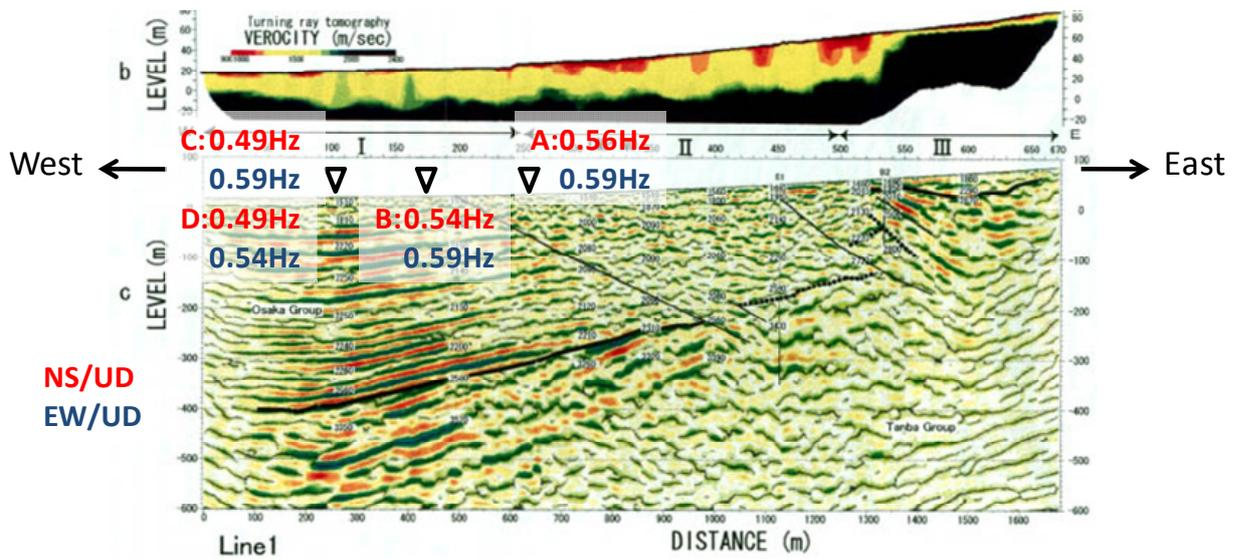
**Figure 2.4.** Section profile beneath Uji campus along the east-west survey line in Fig. 2.5b (After Koizumi *et al.*, 2002) and peak frequencies of average H/V spectral ratios of June 21<sup>st</sup>, 2010, observed at sites A to D in Fig. 2.1b
