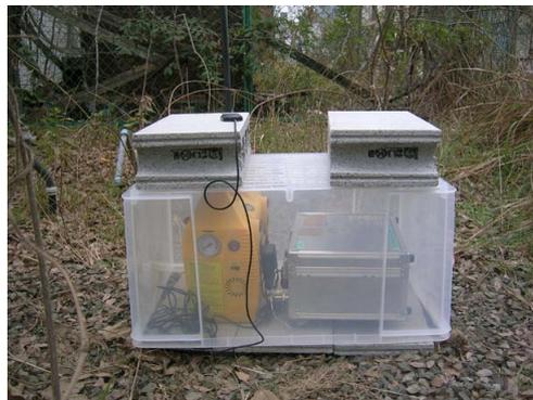
**Photo 2.1.** Example of microtremor measurement site using portable accelerometer SMAR-6A3P and external battery
