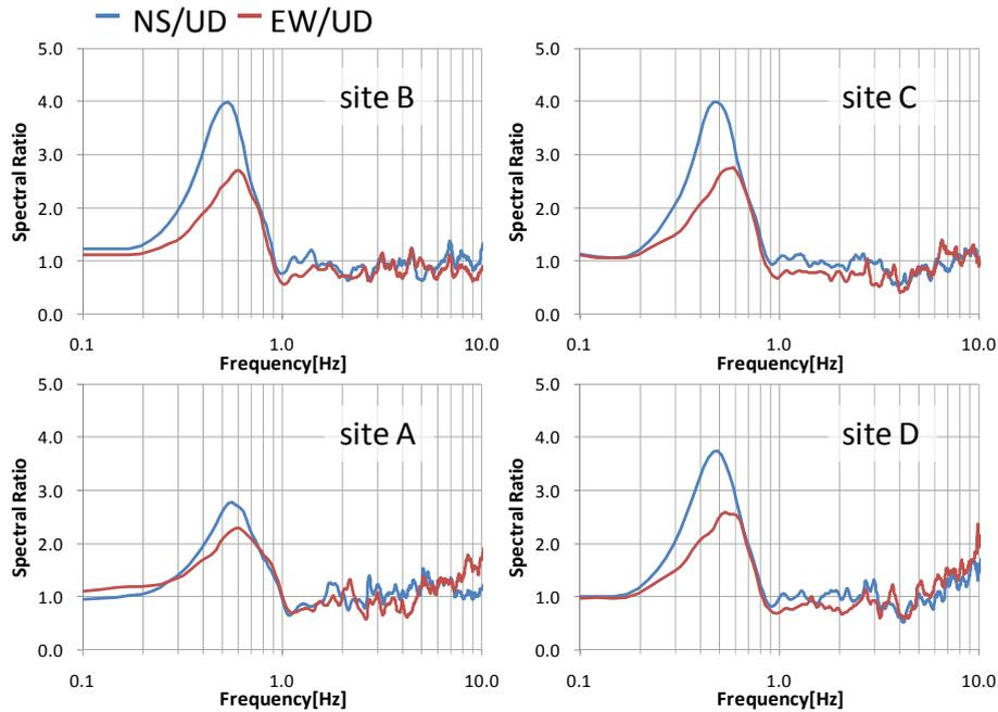
Figure 2.2. Average H/V spectral ratio of June 21<sup>st</sup>, 2010, observed at sites A to D in Fig. 2.1b
