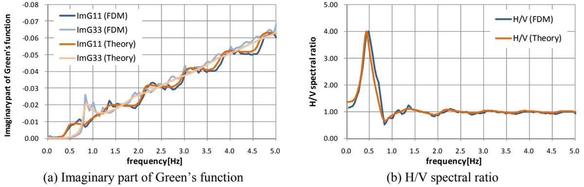
**Figure 4.2.** Comparison of (a) imaginary part of Green's function and (b) H/V spectral ratio of theoretical and numerical results for 1-D velocity model in Table 4.2
