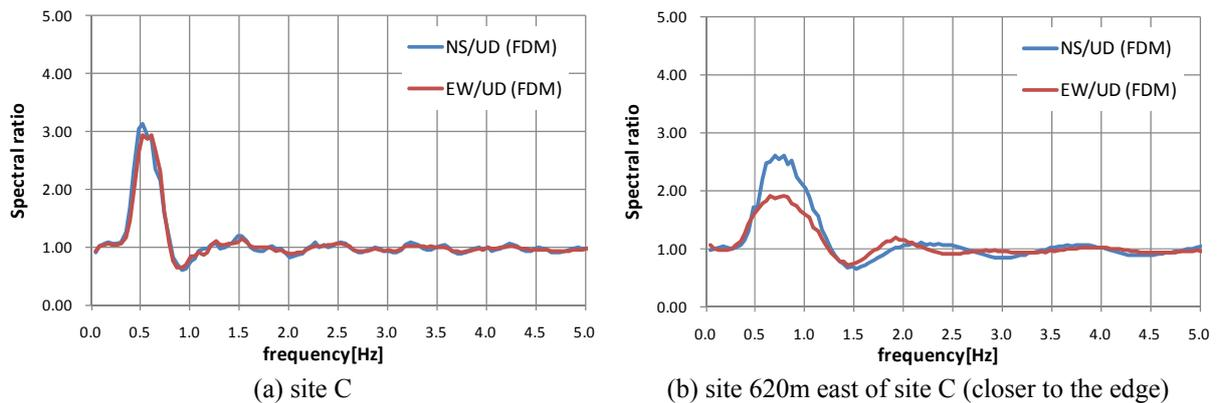
**Figure 4.3.** Comparison of H/V spectral ratio of NS/UD and EW/UD at (a) site C and (b) site 620m east of site C closer to the edge, calculated by FDM for 2-D basin model
