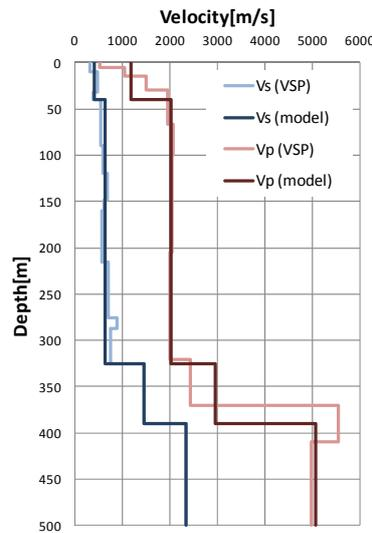
**Figure 3.1.** Velocity profile from VSP survey near site C (light lines) and assumed 1-D velocity model with 3 layers (dark lines)
