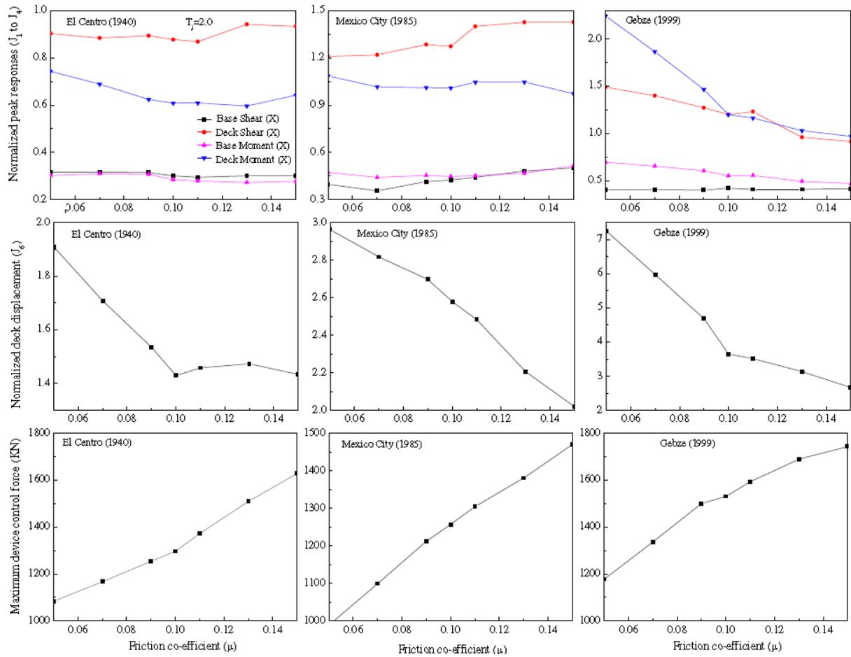
**Figure 5. Effect of friction coefficient of VCFPS on normalized responses of the bridge**
