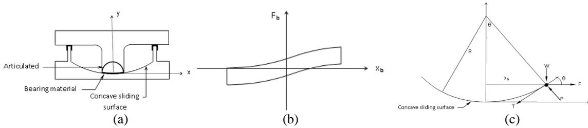
**Figure 3. (a) Schematic diagrams, (b) ideal force-deformation behavior, (c) forces acting on concave sliding surface of VCFPS.**
