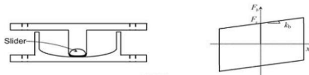
**Figure 2. Friction Pendulum System (FPS)**
