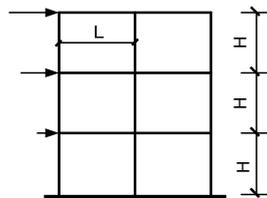
**Figure 3.1.** Sketch of elevation and load pattern
