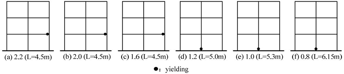
**Figure 4.2.** Location of the first plastic hinge for different  $\beta_c$
