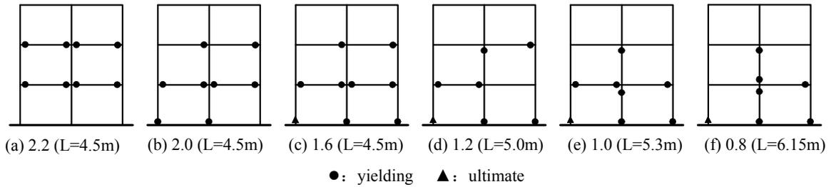
**Figure 4.3.** Comparison of destruction state under top displacement 75mm for different  $\beta_c$
