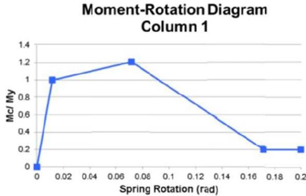
**Figure 5.** Backbone moment-rotation curve of the spring element of a typical column member of the “benchmark” building
