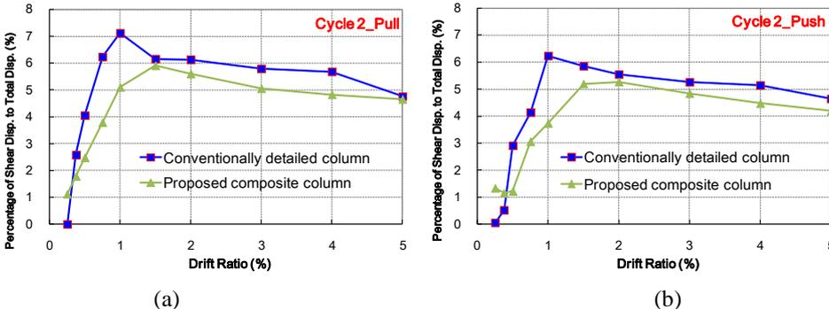
Figure 11. Percentage of shear displacement to the total displacement for the second cycle of cyclic loading which was applied along: (a) the south direction (pull); (b) the north direction (push)
