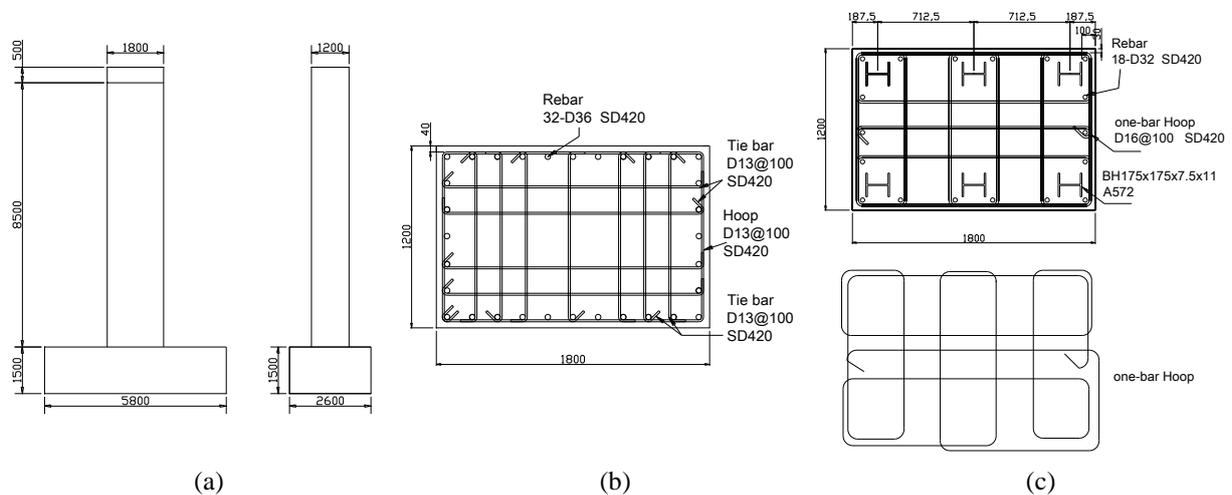
**Figure 1.** Design details of specimen (a) side view of the specimens (b) design details of the conventional column (c) design details of the proposed composite column
