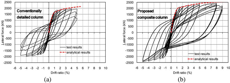
Figure 7. Experimental results (a) conventionally detailed column (b) proposed composite columns
