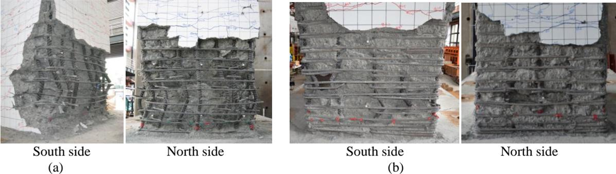
Figure 9. comparison of failure mode (a) conventional pier for drift ratio 5% (b) proposed pier for drift ratio 9%
