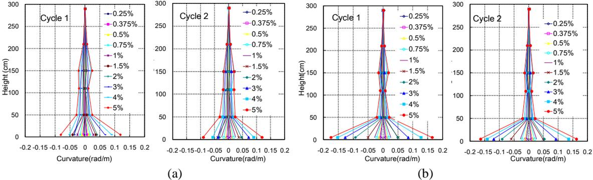
Figure 10. Curvature distributions for different drift ratios (a) conventional pier (b) proposed pier
