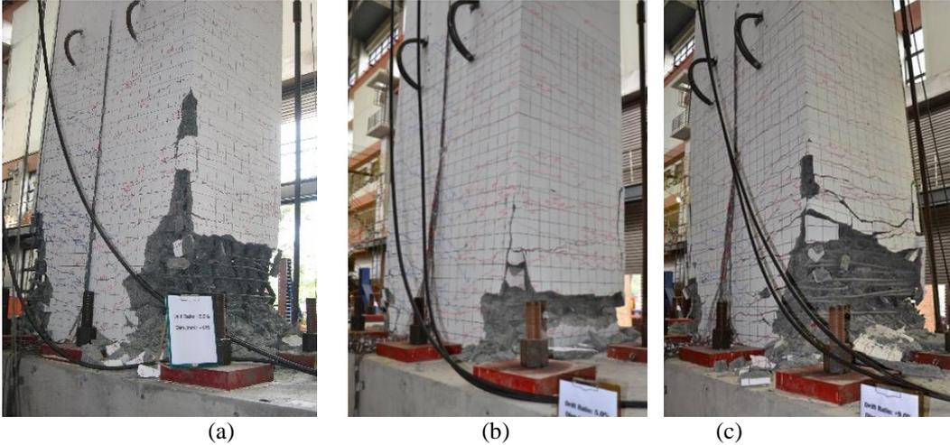
Figure 8. Failure photos for (a) the conventional pier after drift ratio 5% (b) the proposed pier after drift ratio 5% (c) the proposed pier after drift ratio 9%
