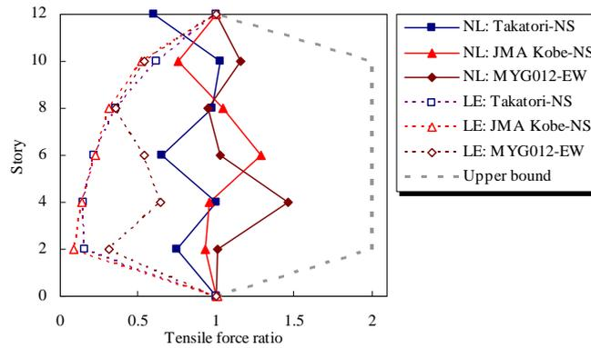
**Figure 3.4.** Maximum horizontal force in BRB connections
