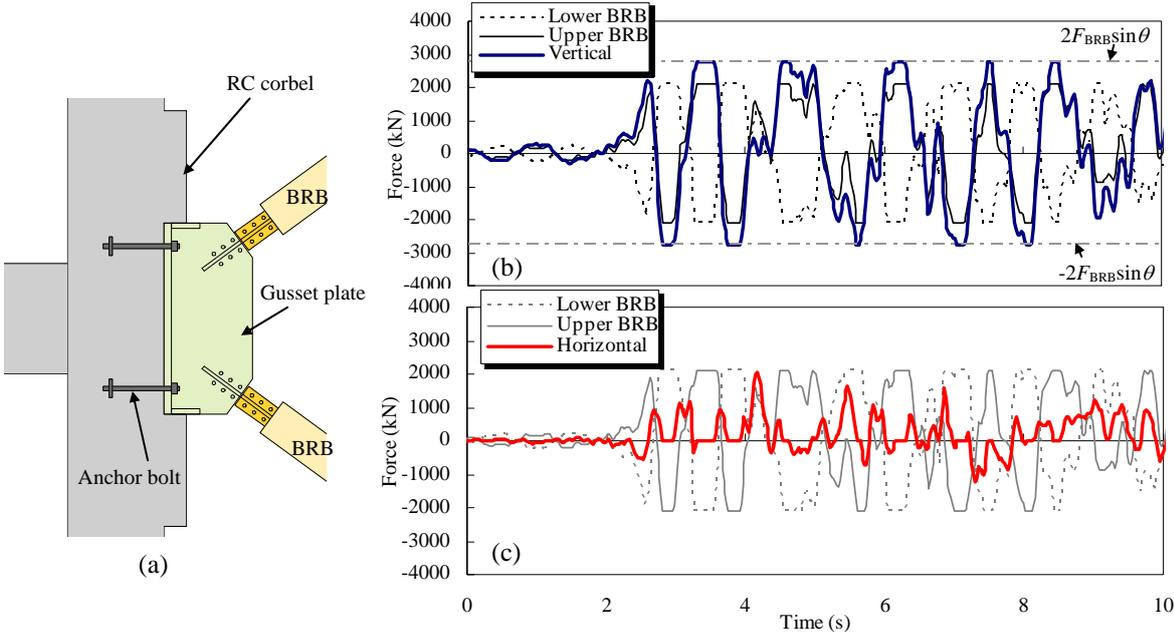
**Figure 3.3.** Force in the BRB connection at 6<sup>th</sup> floor under JMA Kobe-NS: (a) connection detail, (b) vertical component and (c) horizontal component.
