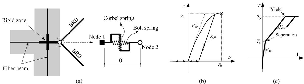
**Figure 4.1.** Modeling of BRB connections: (a) bi-axial spring element, (b) hysteresis of a single corbel and (c) force-displacement relationship of bolt spring
