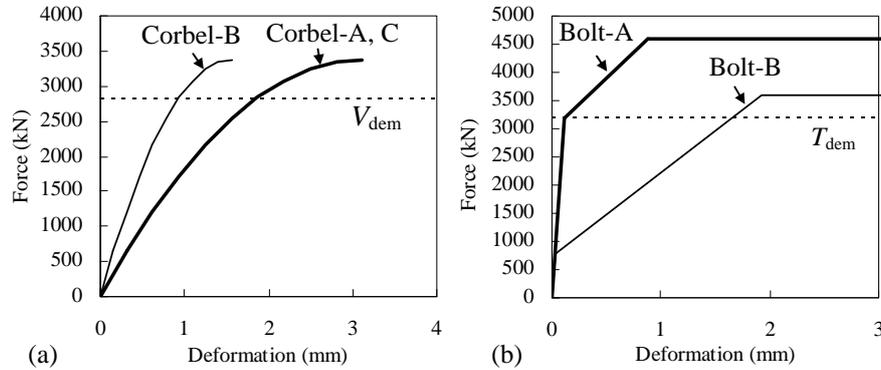
**Figure 4.2.** Models of springs in the BRB connection: (a) corbel models and (b) prestressing bolt models
