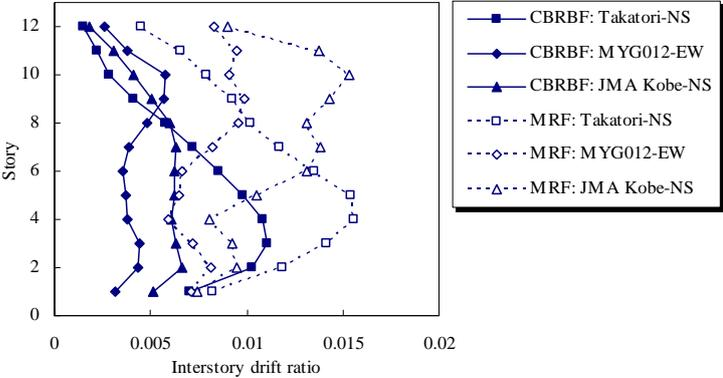
**Figure 3.1.** Maximum interstory drift of moment-resisting frame (MRF) and continuously buckling restrained braced frame
