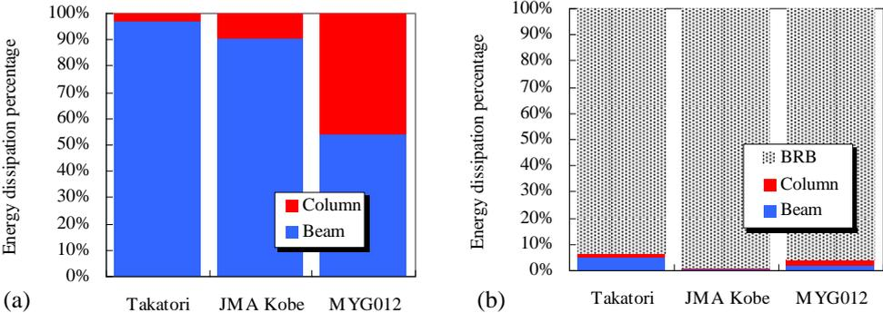
**Figure 3.2.** Hysteretic energy dissipation distributions among different components: (a) moment resisting frame (MRF) and (b) continuously buckling restrained braced frame
