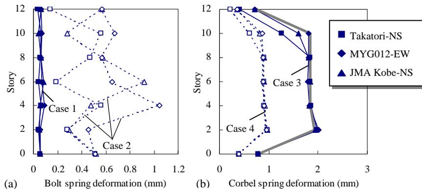
**Figure 4.3.** Maximum bolt spring deformations
