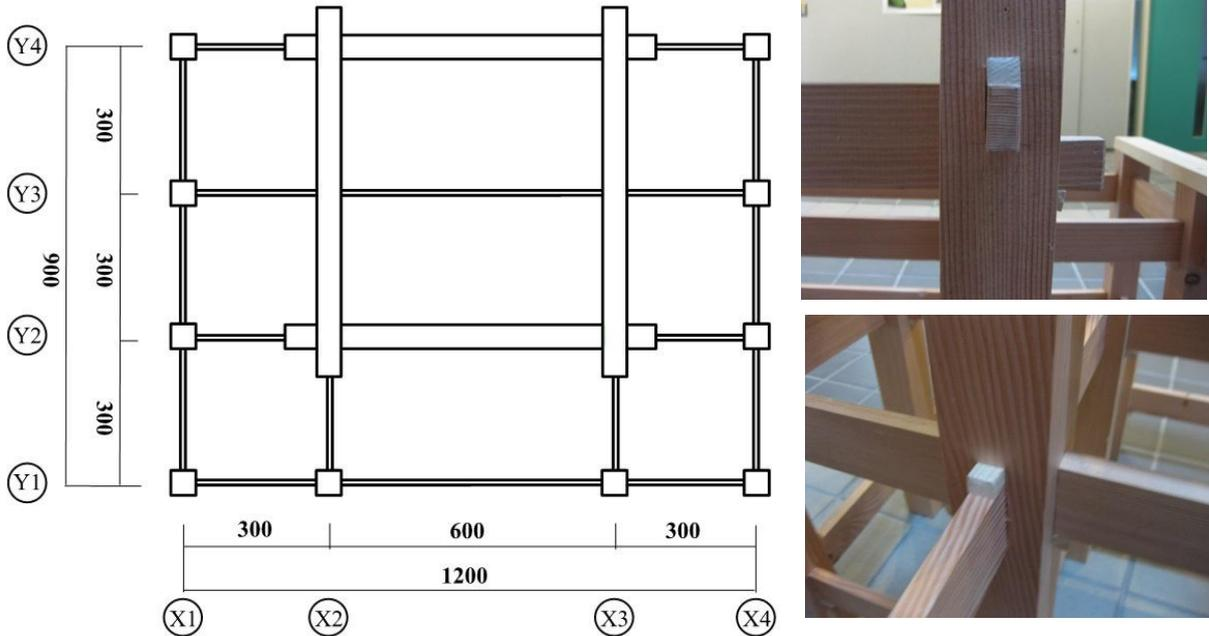
Figure 2. Dimension of the model and joint details
