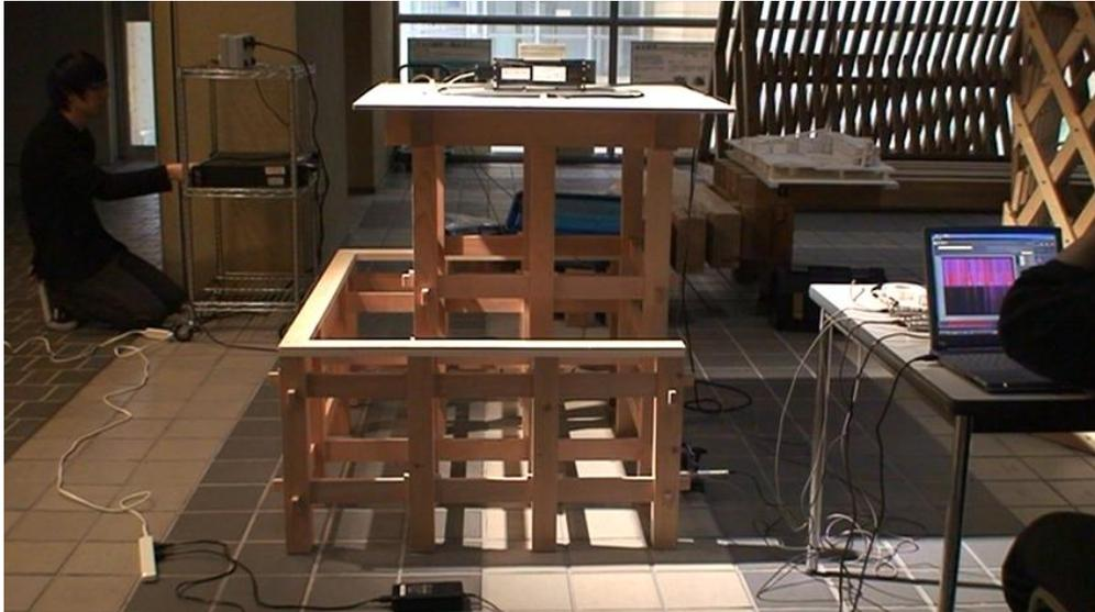
**Figure 4.** General layout of the forced vibration test
