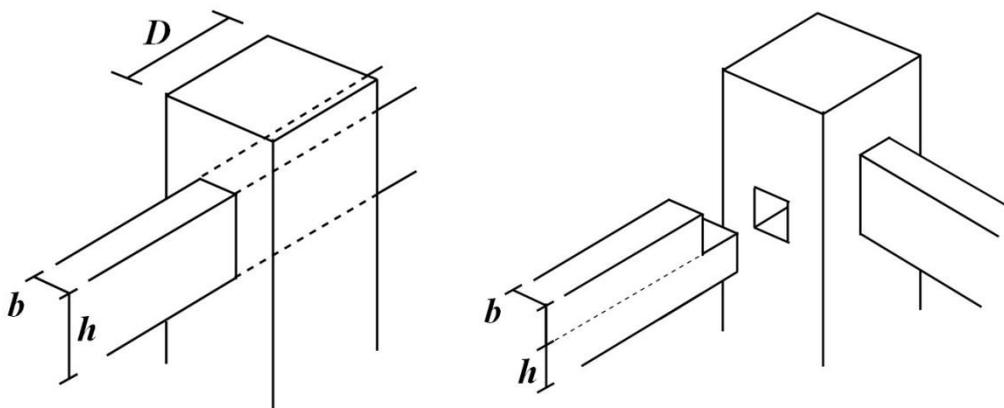
**Figure 6.** Types of tenon joints for the model
