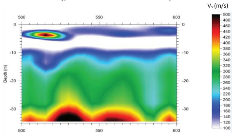
Figure 5.3: MASW data taken along Park Terrace indicating presence of an infilled channel
