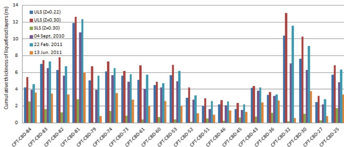
Figure 6.2. Estimate of liquefied layer thicknesses for different seismic events
