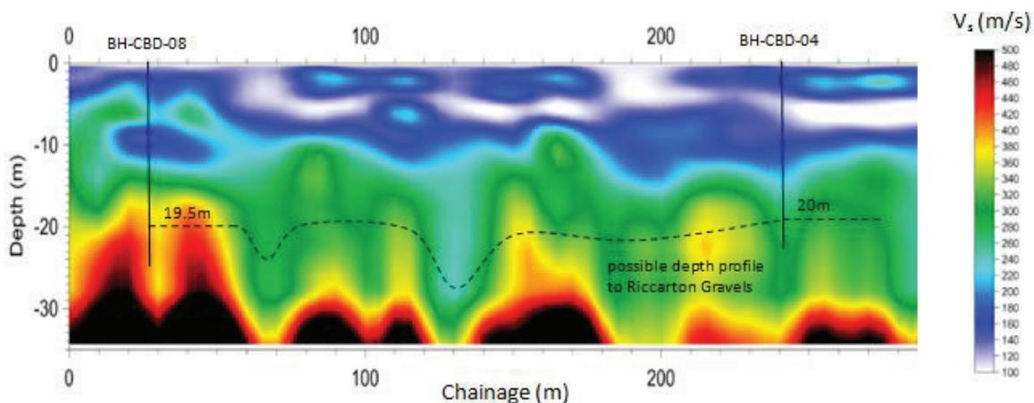
Figure 5.4: Depth to Riccarton Gravels indicated by machine boreholes and inferred from MASW
