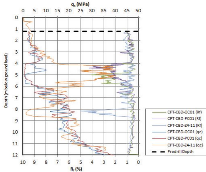
Figure 5.2. Piezocone calibration plots
