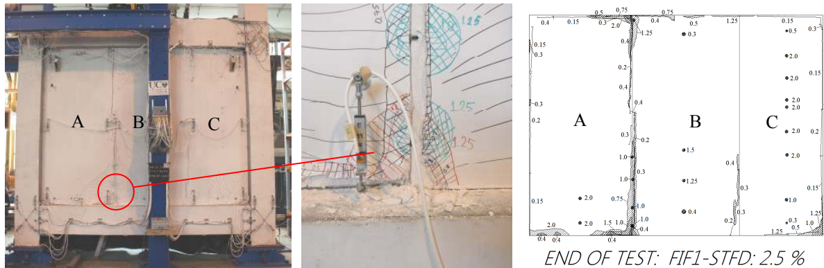
Figure 9. Damage state of steel framed drywall FIF1-STFD at the end of test
