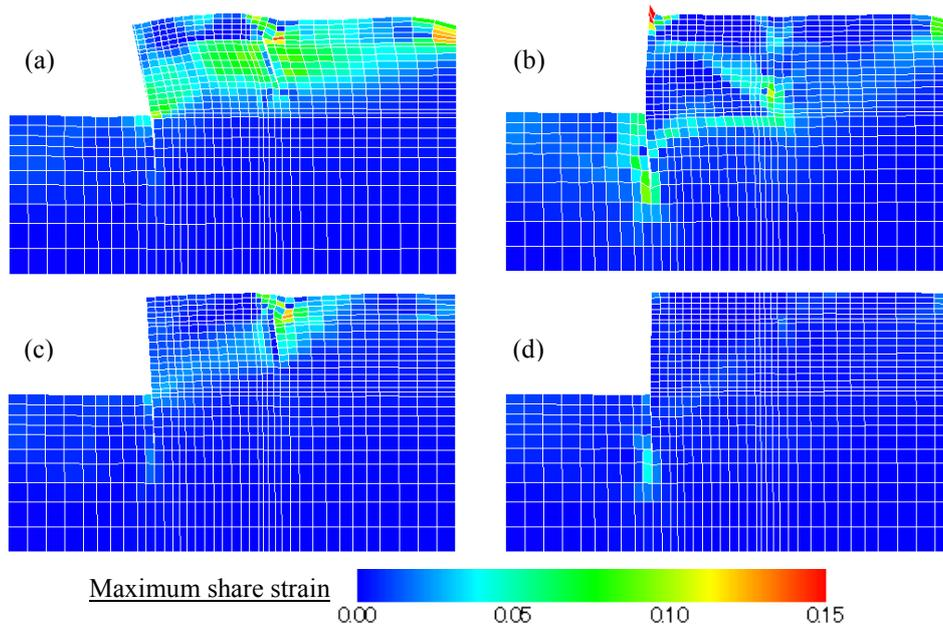
**Figure 6.** Computed permanent deformation (Displacement magnification: 5 times) and distribution of maximum shear strain: (a) Case-A1, (b) Case-A2, (c) Case-A3, (d) Case-A4
