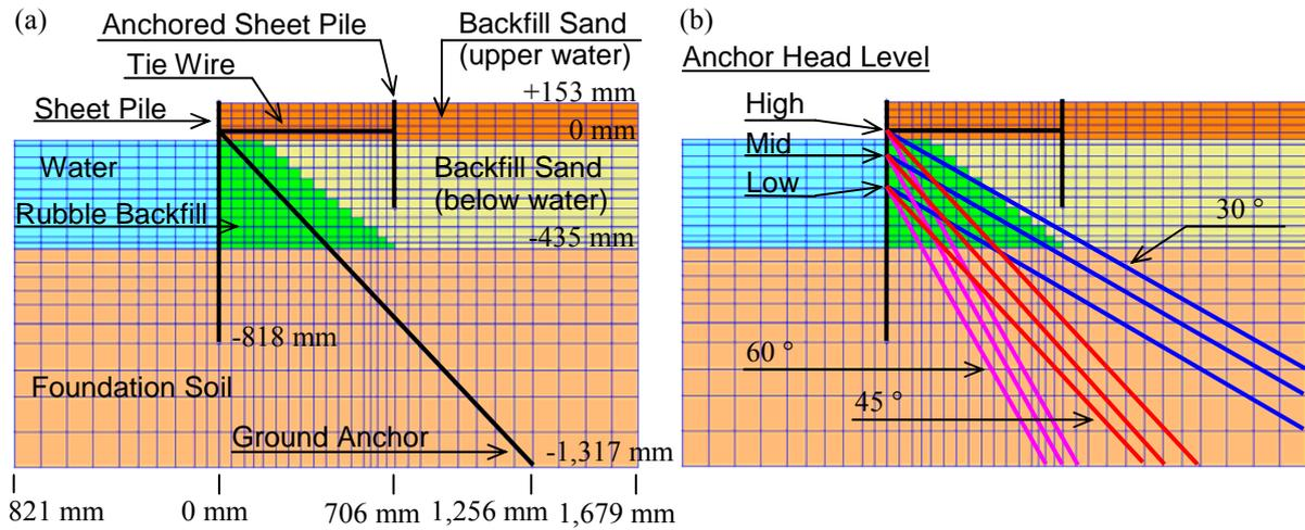
**Figure 3.** Finite element mesh for analysis: (a) Analysis of liquefiable condition of backfill sand (Series A); (b) Analysis of arrangement of ground anchors (Series B)
