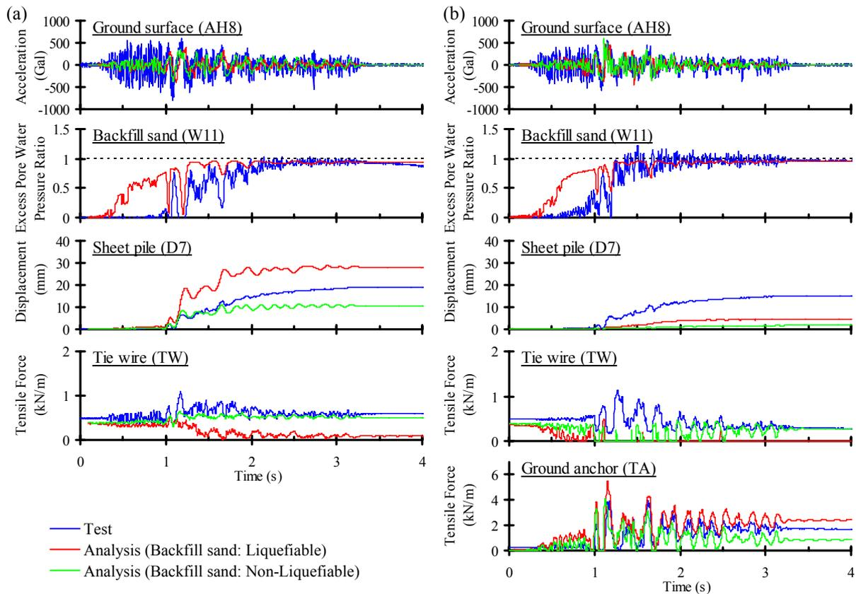
**Figure 4.** Comparison of time histories obtained by the test and the analysis: (a) Without ground anchor, (b) With a ground anchor
