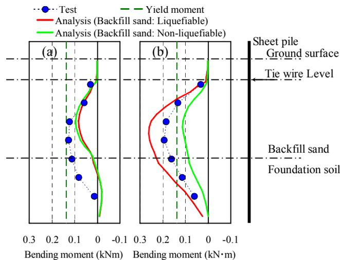
**Figure 5.** Comparison of distribution of maximum bending moment of sheet pile obtained by the test and the analysis: (a) Without ground anchor, (b) With a ground anchor
