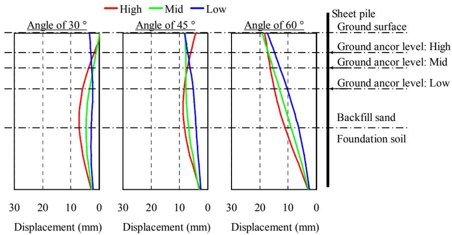
**Figure 7.** Computed distribution of permanent displacement of sheet pile by arrangement of ground anchor
