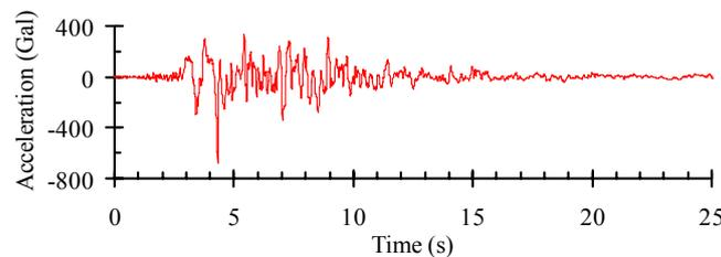
**Figure 2.** Input strong motion record (prototype)
