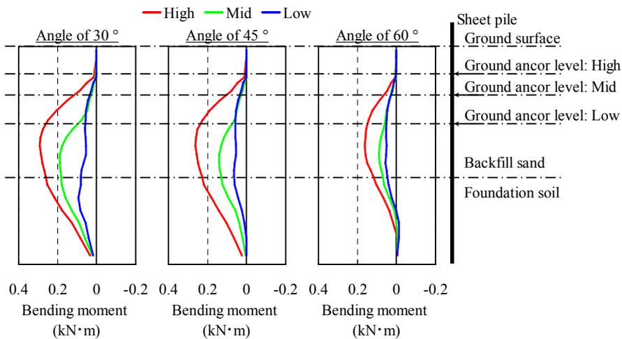
**Figure 8.** Computed distribution of maximum bending moment of sheet pile by arrangement of ground anchor
