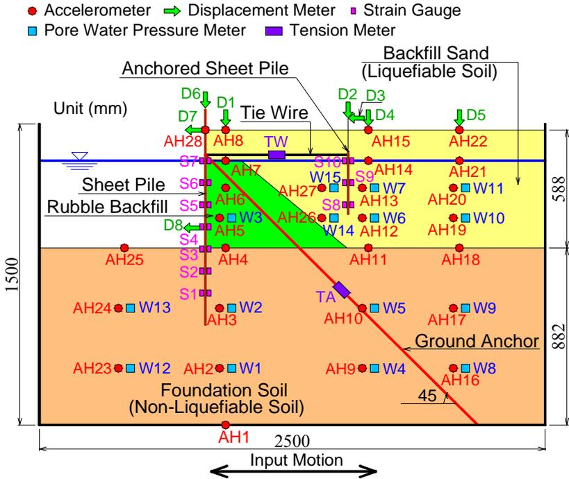
**Figure 1.** Cross section of test model
