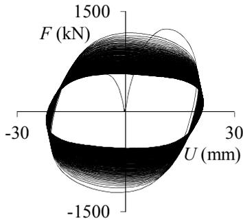
Figure 10. Hysteresis curve of standard condition
