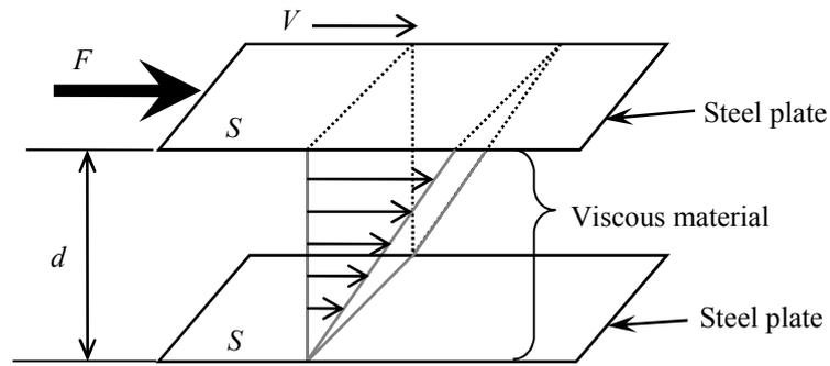
**Figure 1.** Mechanism of damping force
