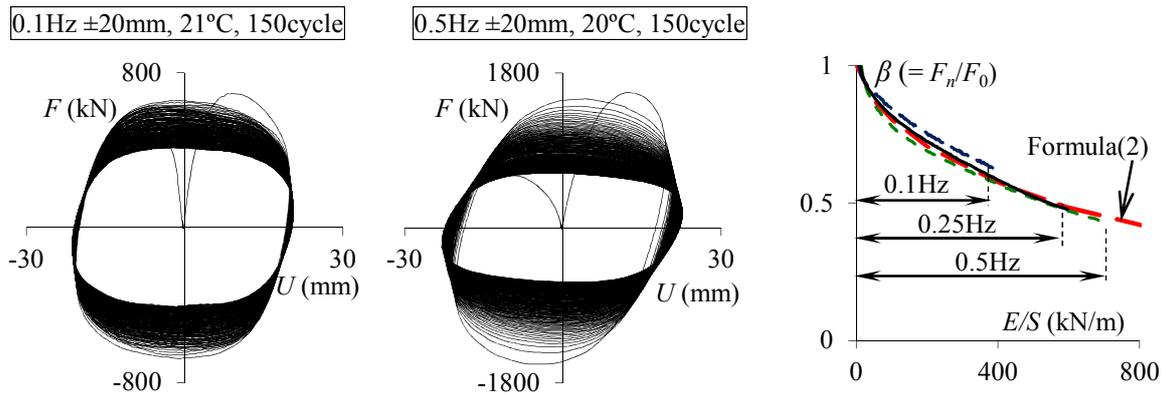
Figure 14. Differences between frequency 0.1, 0.25 and 0.5Hz
