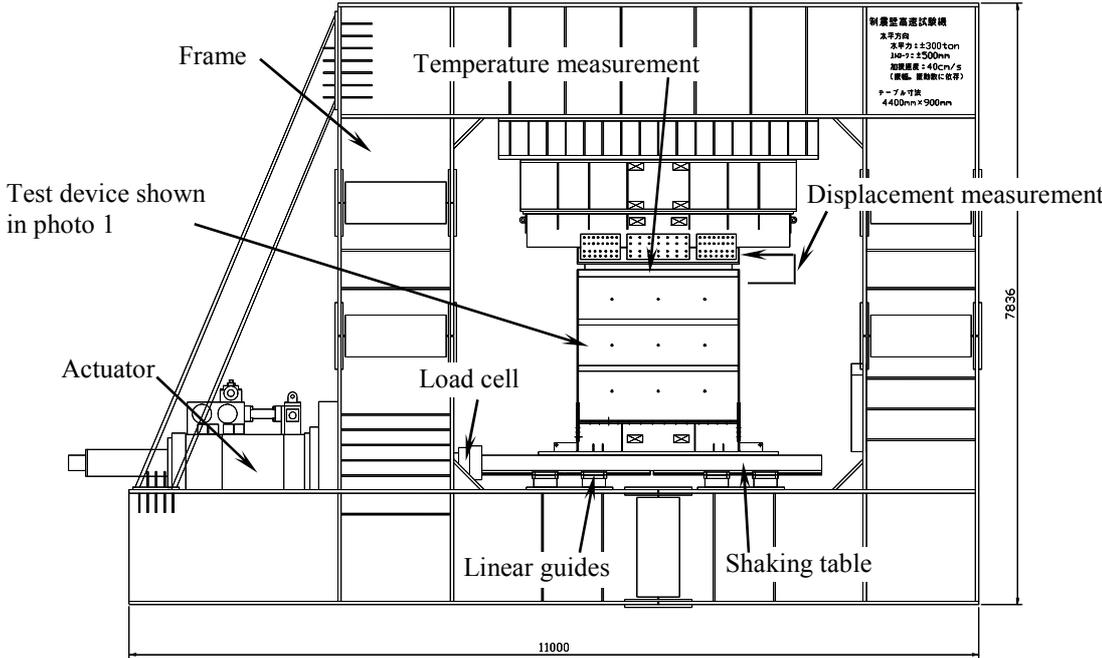
Figure 4. Test apparatus, test device and measurements
