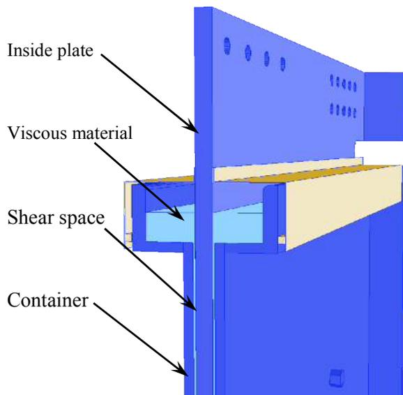
**Figure 2.** Structure of the damper
