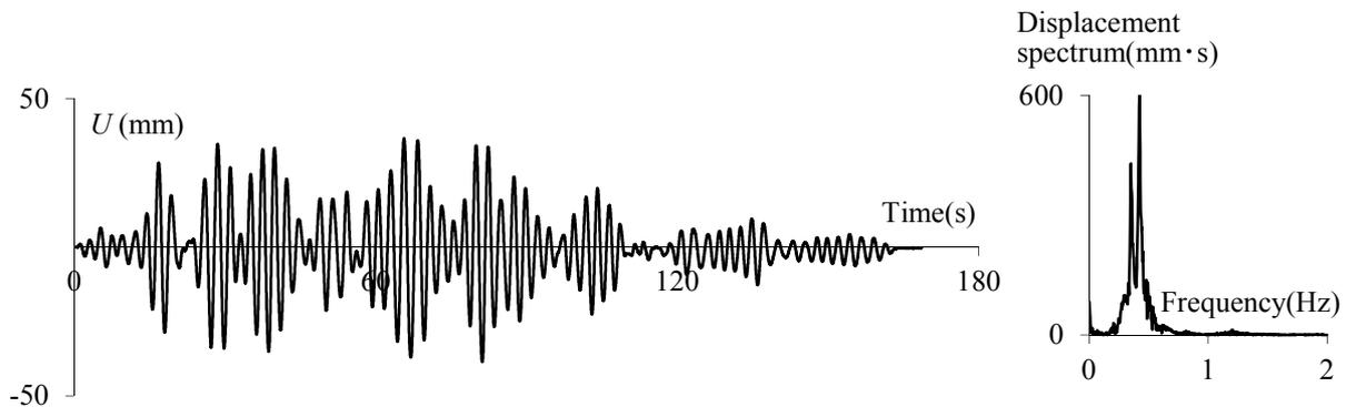
Figure 16. Displacement of random wave time history and spectrum
