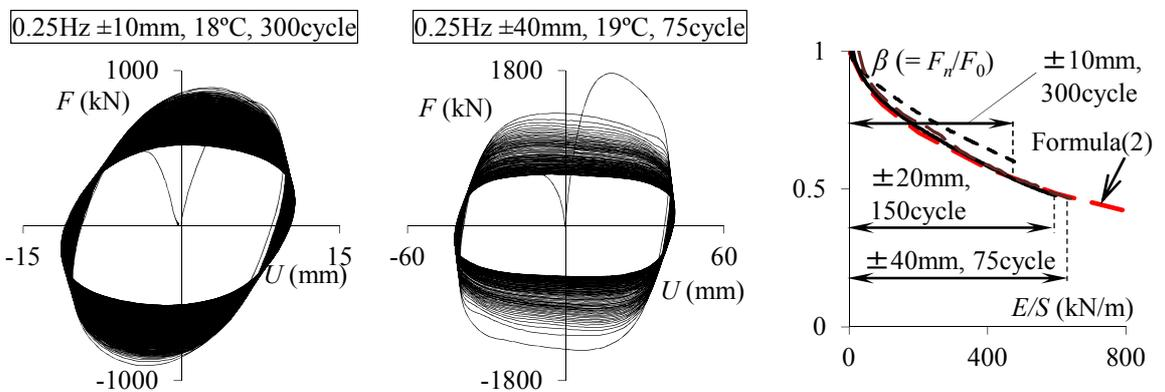
Figure 15. Differences between amplitude ±10mm300cycle, ±20mm150cycle and ±40mm75cycle
