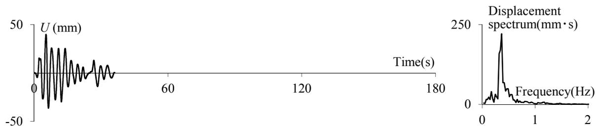
Figure 7. Displacement time history and spectrum of random wave
