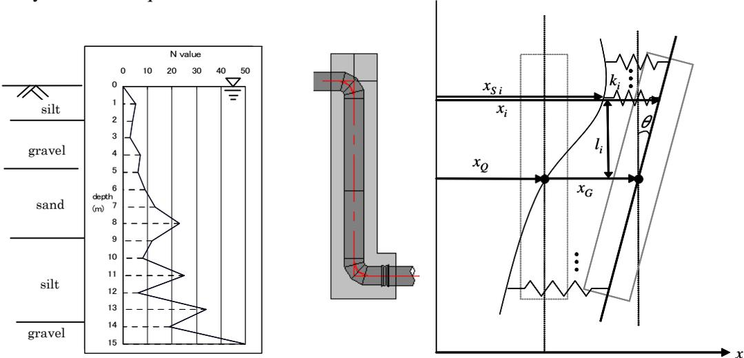
Figure 3.11. Soil classification and N value at site Figure 3.12. Configuration of the coordinate system for riser
