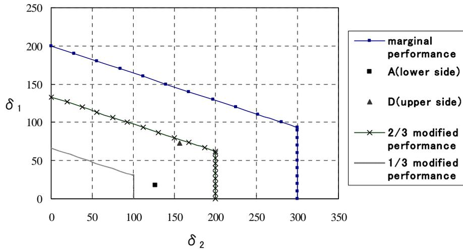
**Figure 3.6.** Multiple limit state diagram of expansion joint failure modes, in which modified performance curves are generated from the marginal performance curve in deteriorated joint allowance states
