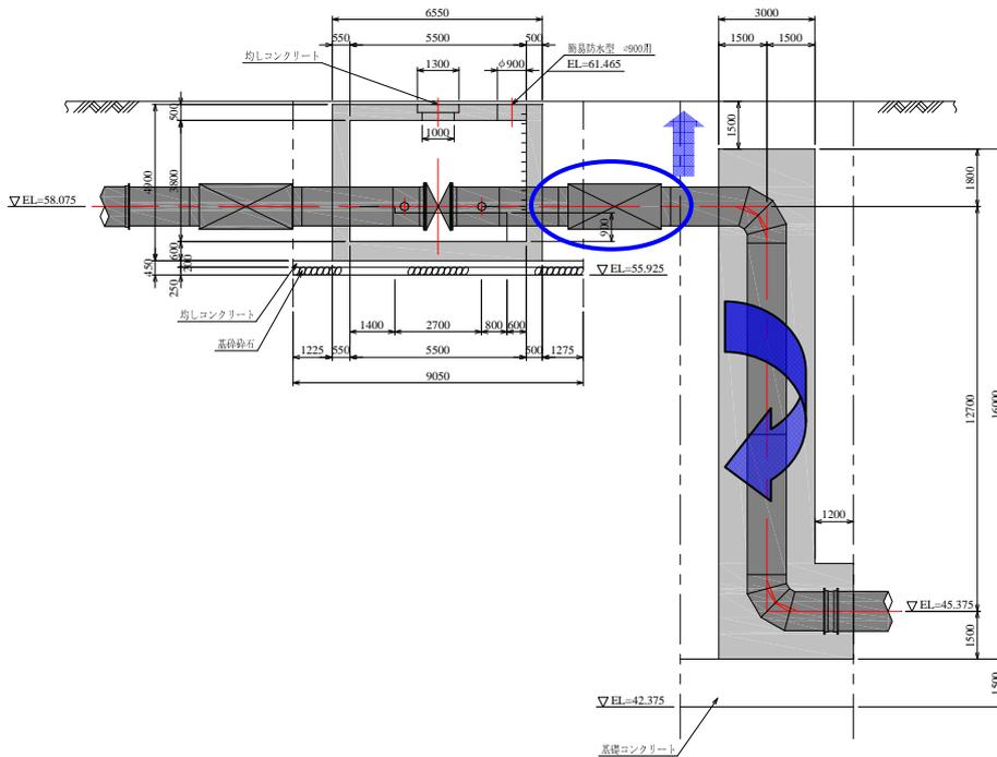
Figure 3.9. Schematic illustration of riser and valve pit system
