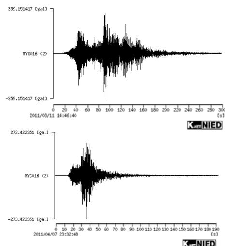
**Figure 2.2.** Strong ground motion at Shiroishi (MYG016) in main shock (2011.3.11) and after shock (2011.4.7)
