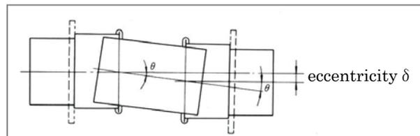
**Figure 3.14.** Allowable angle of expansion joint for eccentricity  $\delta$
