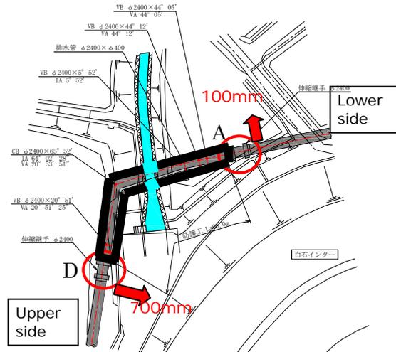
Figure 3.1. Location map of expansion joints under-crossing stream line
