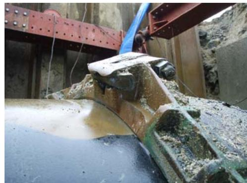
**Photo 3.3.** Sealing bolt worn out by hydro-blasting
