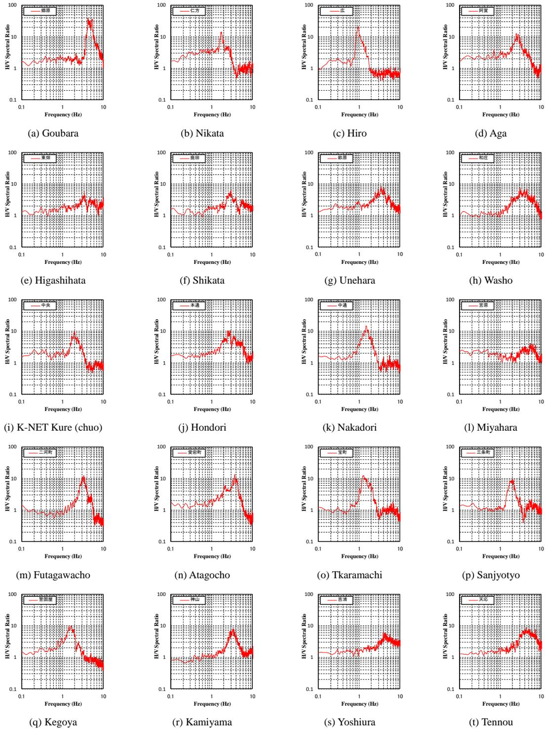
**Figure 10.** The observed H/V spectrum at each site
