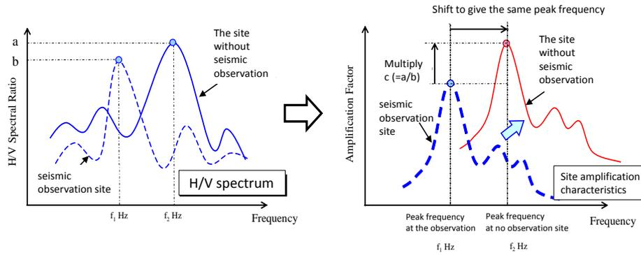
**Figure 4.** Schematic illustration of the applied correction procedure
