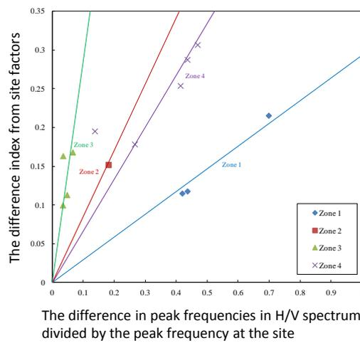
**Figure 6.** The relationship between the difference in corrected site factors and the difference in peak frequencies of microtremor H/V spectrum
