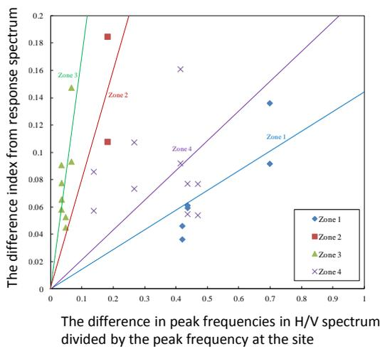
**Figure 5.** The relationship between the difference index of estimated motions and the difference in peak frequencies of microtremor H/V spectrum
