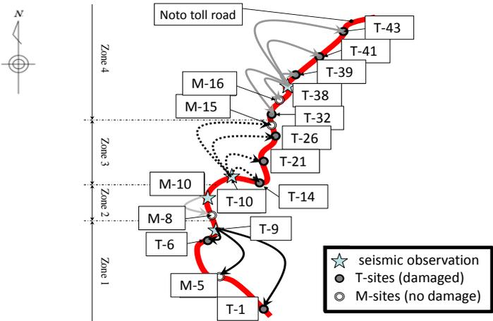
**Figure 3.** The pair of the sites for the correction of site amplification characteristics<sup>3)</sup>
