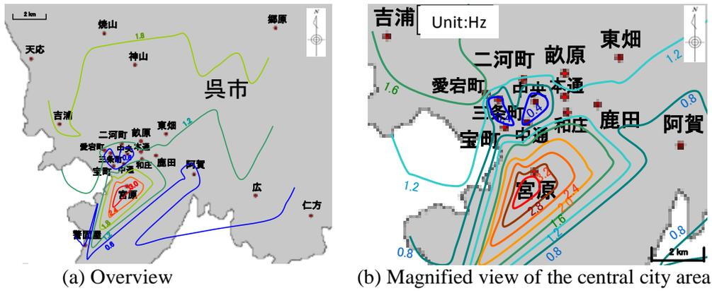
**Figure 11.** The contour of the difference in peak frequency of H/V spectrum of each site from that of the K-NET Kure site
