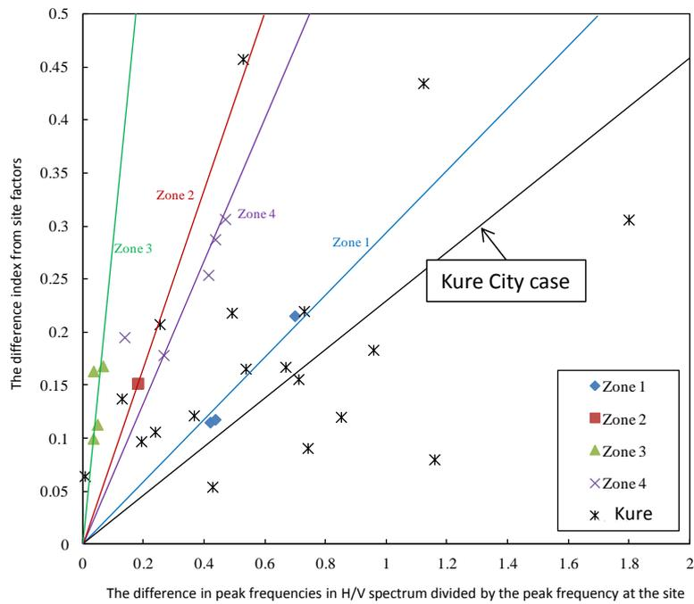
**Figure 12.** The relationship between the difference indexes of corrected site amplification factors and the difference in peak frequencies of microtremor H/V spectrum for Kure City case
