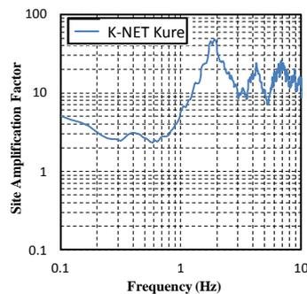
Figure 9. Site amplification factor at K-NET Kure site<sup>5)</sup>
