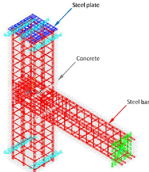
**Figure 2.4.** The FE model of a typical exterior beam-column sub-assembly
