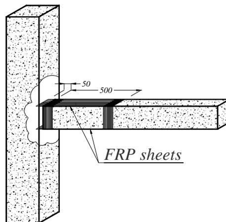
**Figure 2.6.** Retrofitting configuration in order to relocate plastic hinge away from column
