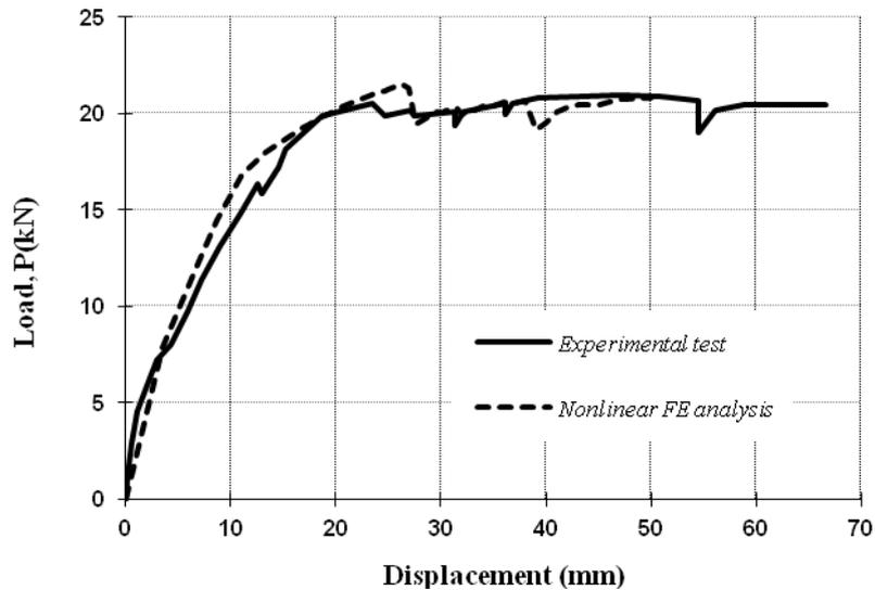
Figure 2.2. Comparison of load-displacement curves for specimen RSM2.
