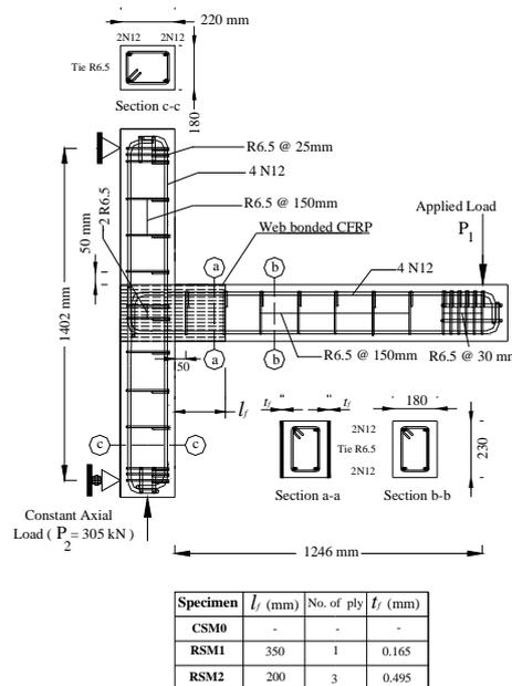
**Figure 2.1.** The CFRP retrofitted beam-column joint tested by Mahini and Ronagh (2011)
