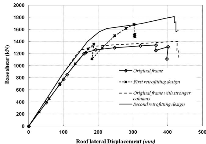
Figure 3.1. Comparison of pushover curves of the original and the retrofitted frames
