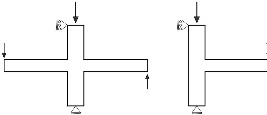
**Figure 2.5.** Schematic illustration of separated joints and applied loads in FE modelling
