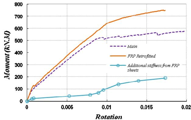
**Figure 2.7.** Moment-rotation curves of the original and the retrofitted exterior joint at the first story
