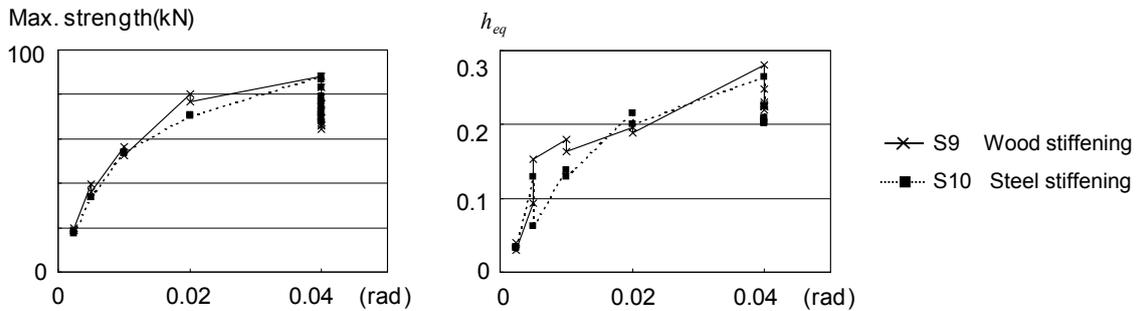
Figure 7. Maximum strength and equivalent damping ratio of S9 and S10
