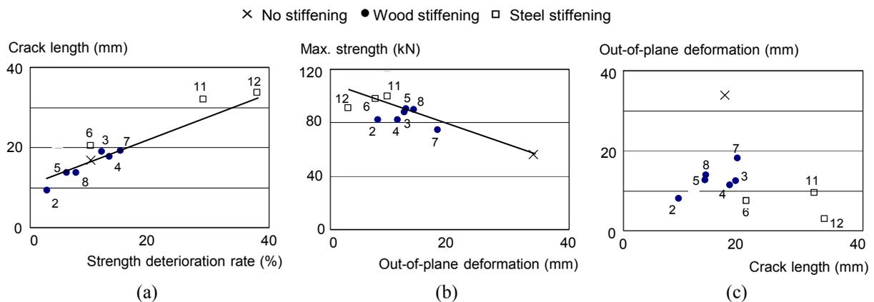
Figure 8. Influences of out-of-plane deformation of steel plate and crack on hysteretic behavior
