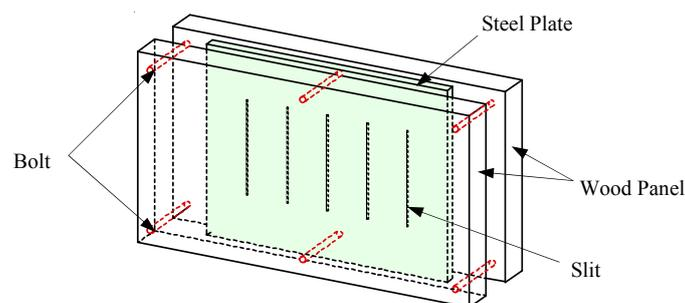
**Figure 1.** Slitted steel shear wall stiffened by wood panels
