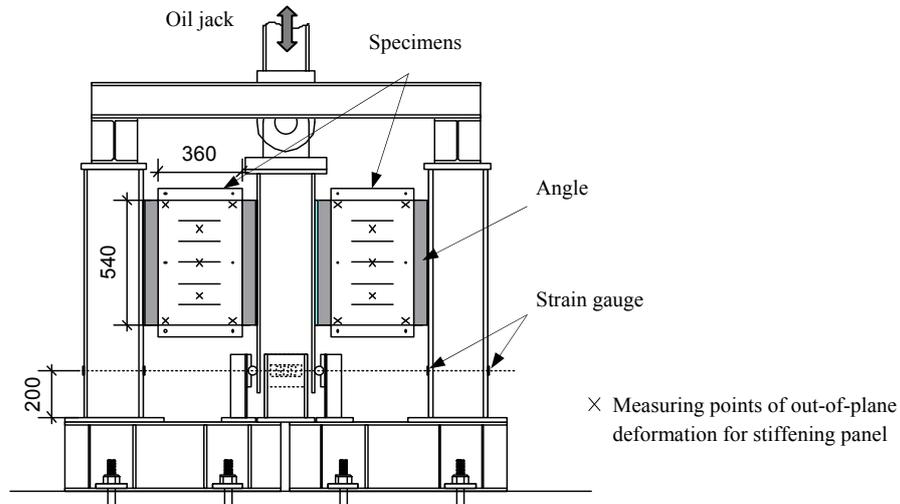
**Figure 3.** Loading setup used in test
