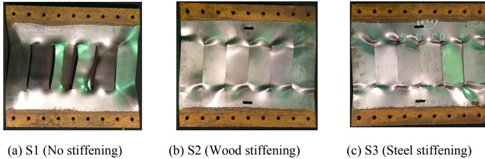
Figure 6. Slitted steel plates after loading
