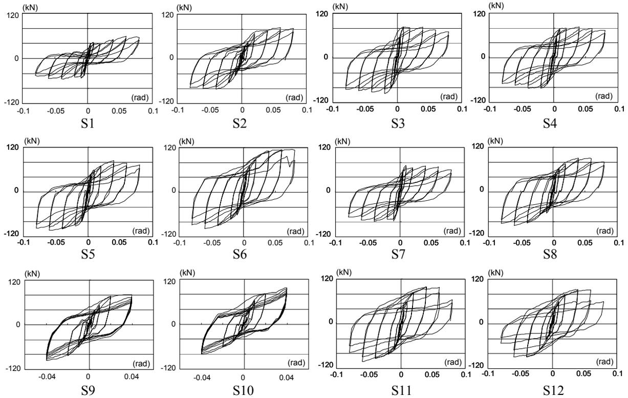
**Figure 4.** Hysteretic loops obtained from tests
