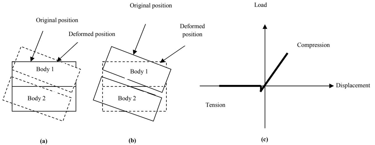
**Figure 4** a. Separation or debonding at interface
