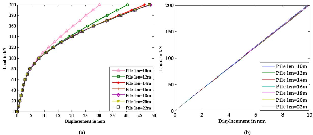
**Figure 7.** Response of single socketed pile for plastic soil case of very soft clay for varying lengths of pile
