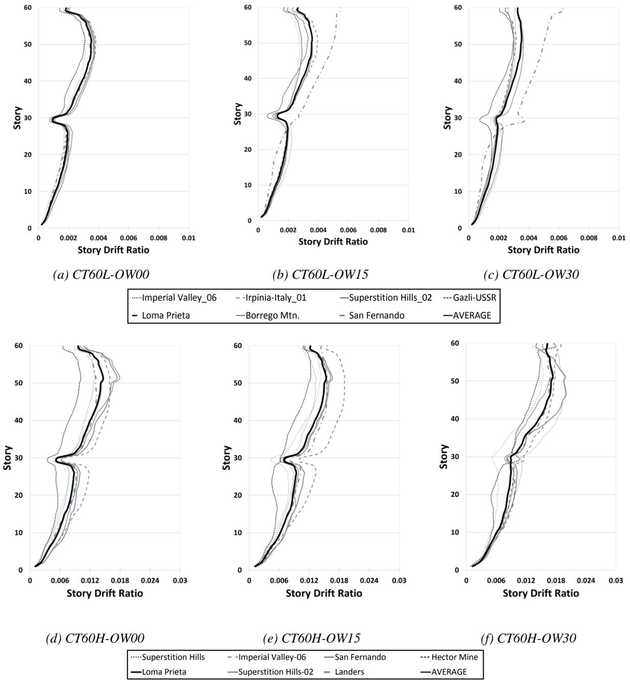
**Figure 5.** Story drift ratio of CT60L-(a, b and c) and CT60H- (d, e and f) after NLRH
