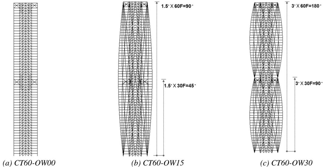
**Figure 2.** Outrigger System configurations**Table 5.** Maximum Drift (CT60L, Boston) and inter-story drift ratio (CT60H, LA)
