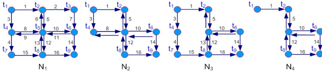
Figure 3. Reduced transportation networks resulting from failures in power and communication networks
