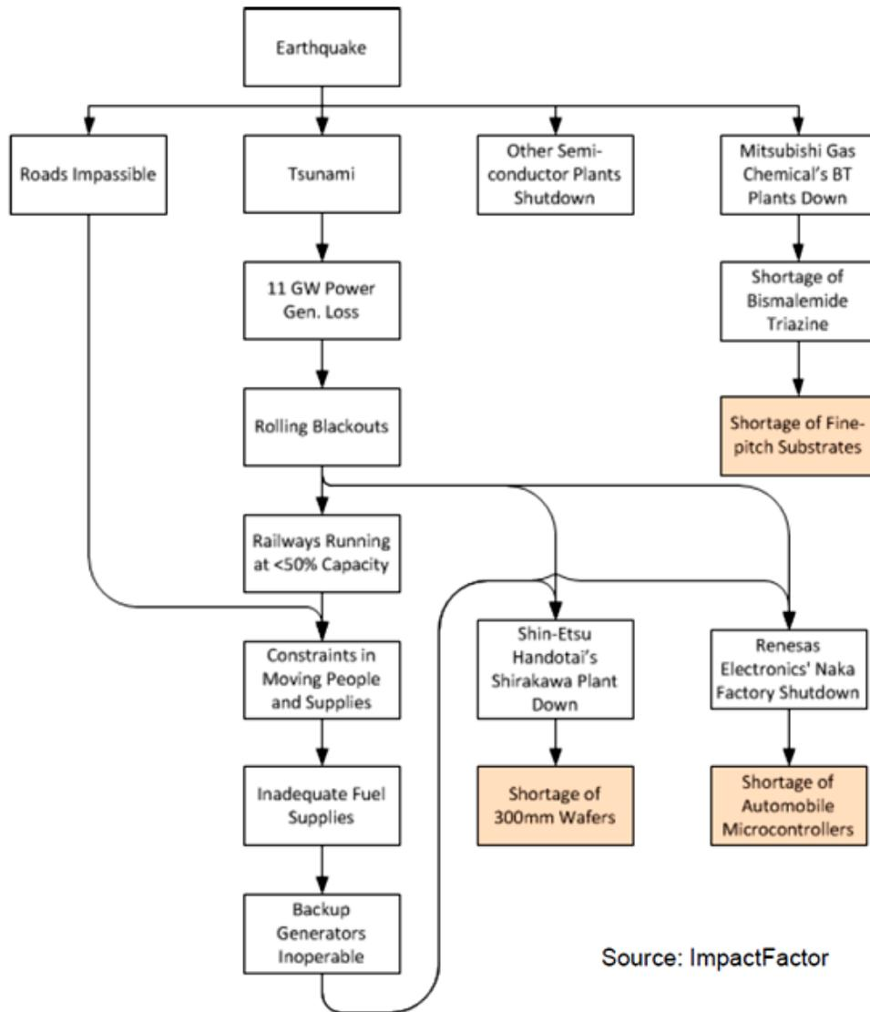
**Figure 1.** Effects of infrastructure failures on supply chain disruptions (ChainLink Research & ImpactFactor, 2011)
